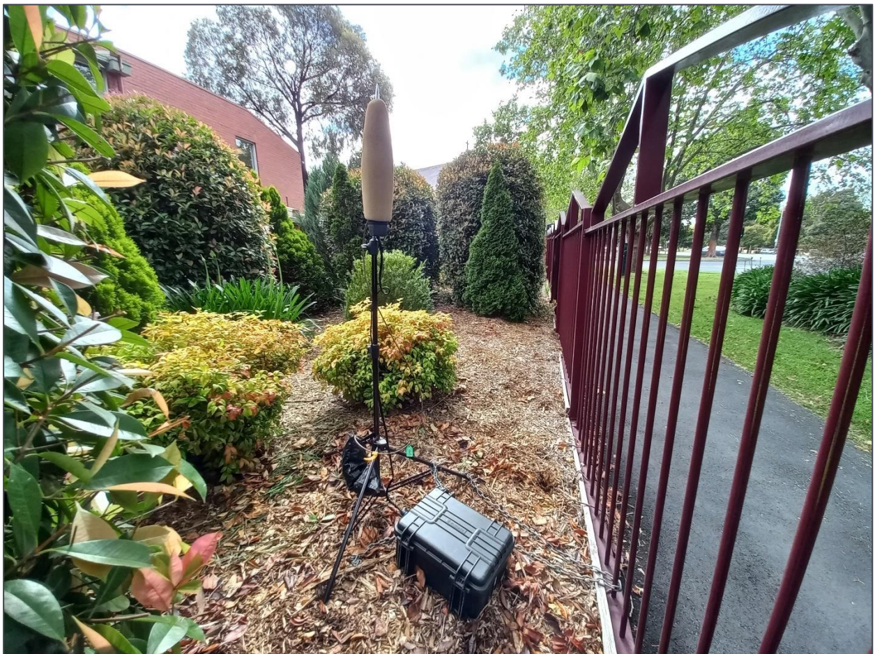
Figure 5: Photograph of noise monitor setup
