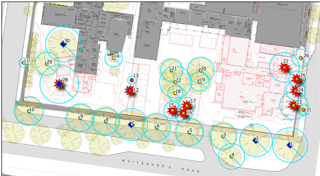
Figure 3. Extract of demolition plan with trees overlaid. Trees colour coded by arb rating: Blue diamonds = High, Green circle = Mod.A, Yellow circle = Mod.B, Orange circle = Mod.C, Red Circle = Low. Light blue circles = TPZs. Red stars = intent to remove.
