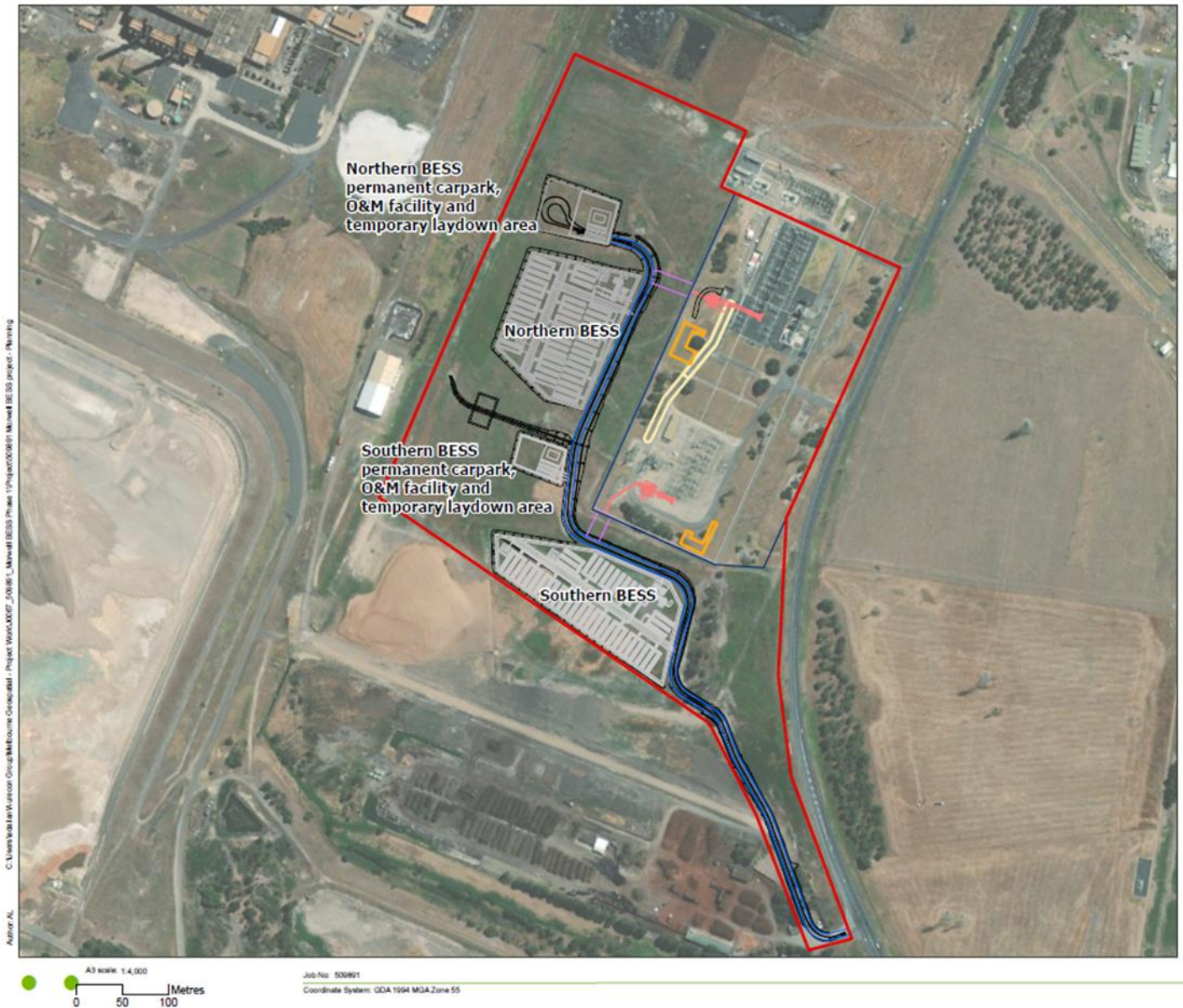
Figure 1-1: Concept design site layout for Latrobe Valley BESS
