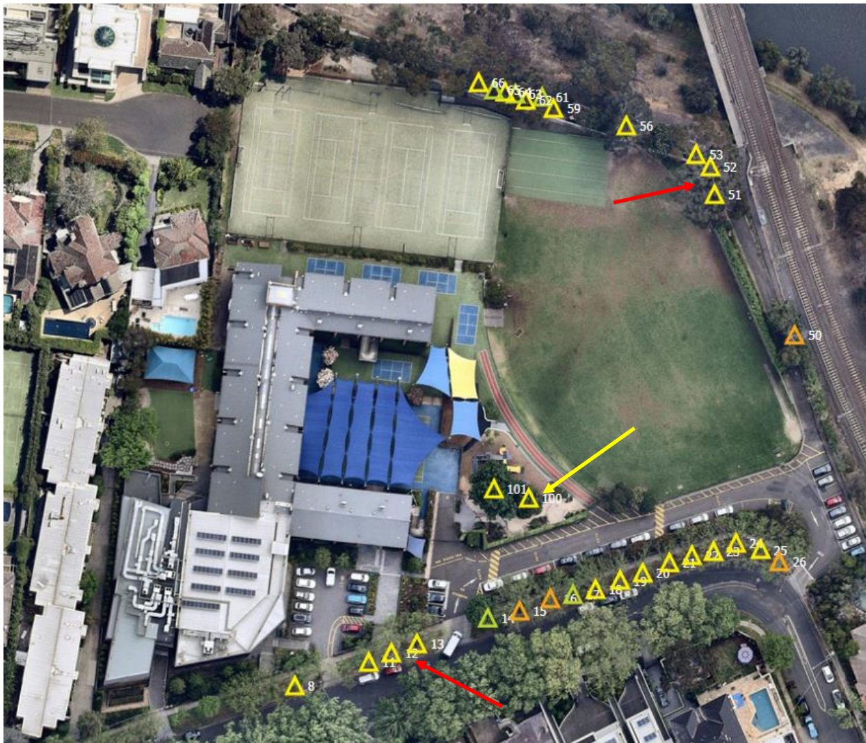
Figure 7. Aerial image showing location of Moderate Retention Value Trees. The red arrows identify 6 x trees recommended for retention with specific protection measures. The yellow arrow identifies 1 x tree that cannot be retained under the current proposal. (ArborPlan, September 2019).
