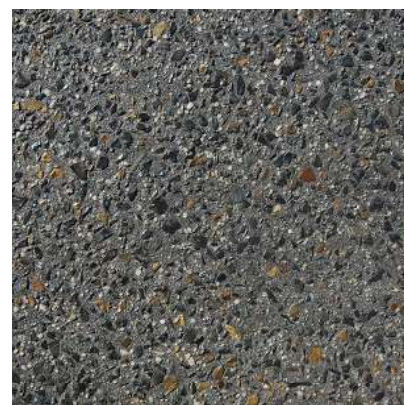
DRIVEWAY Stipple finish concrete paving Charcoal or similar
