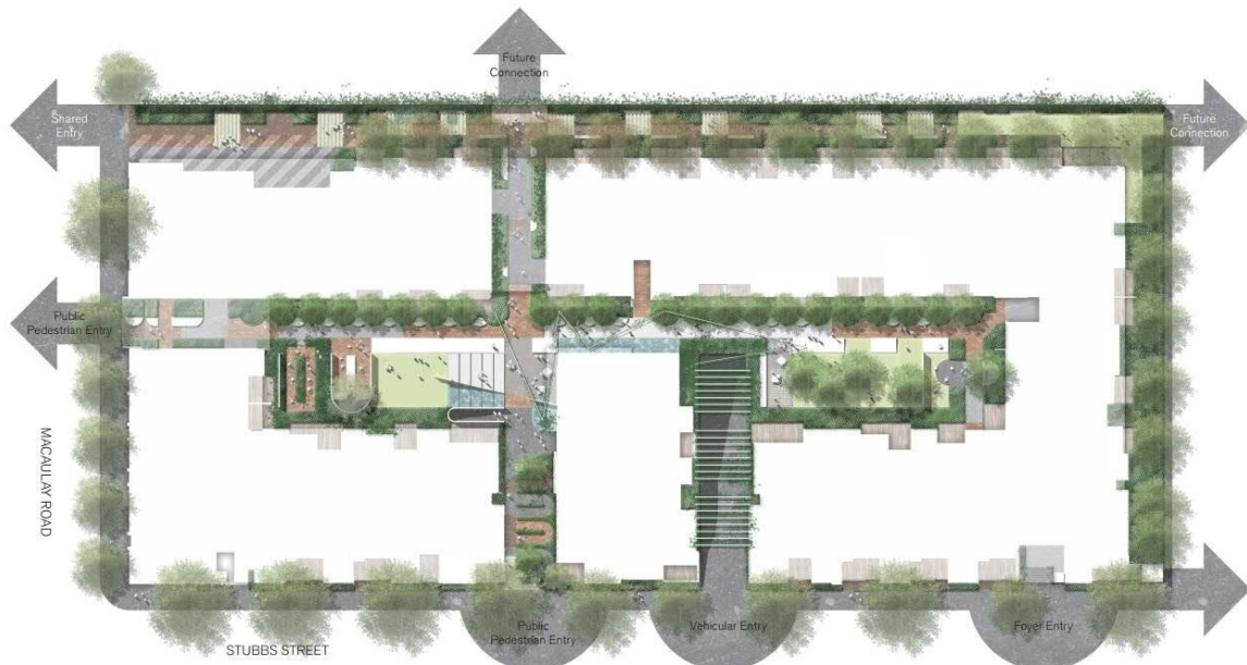
Figure 25: Landscape concept plan that shows the permeability along and across the site, Openwork
