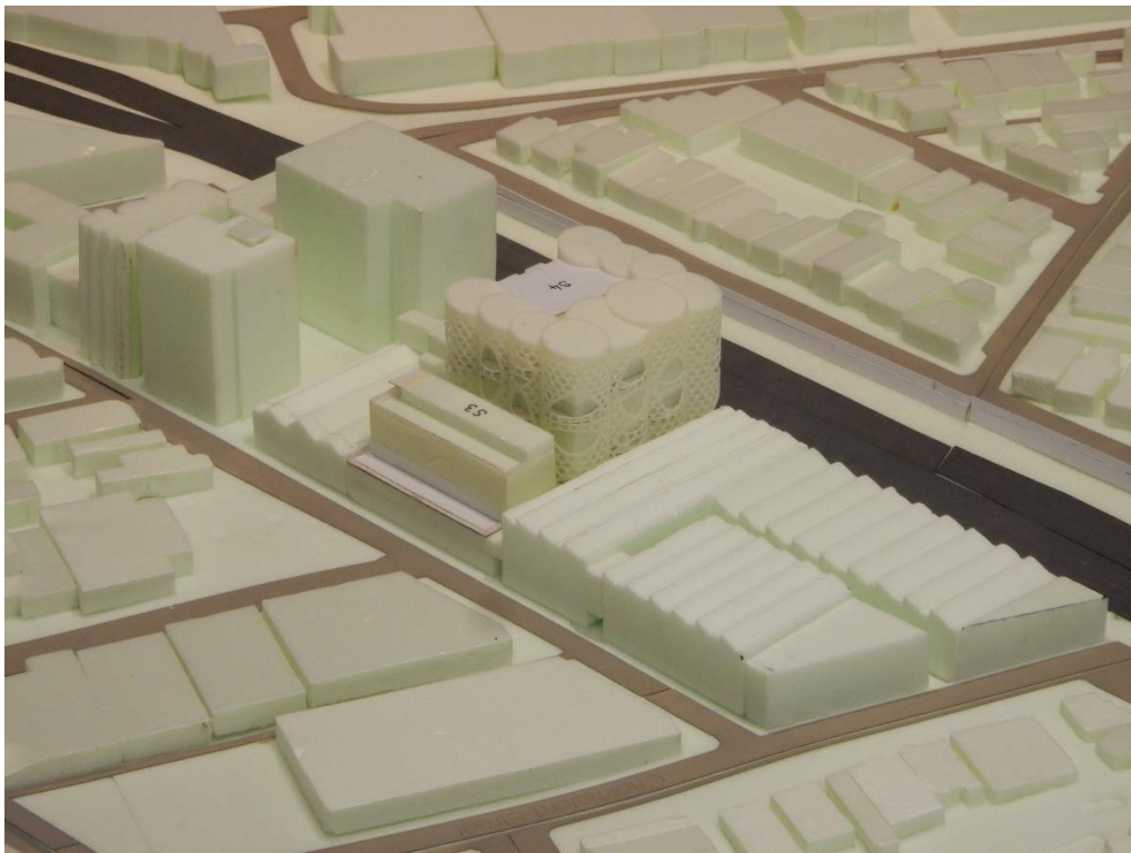
Figure 4 – Close-up view from the northeast of the 1/400 scale proposed Young Husband Stage 2 development in the wind tunnel.
