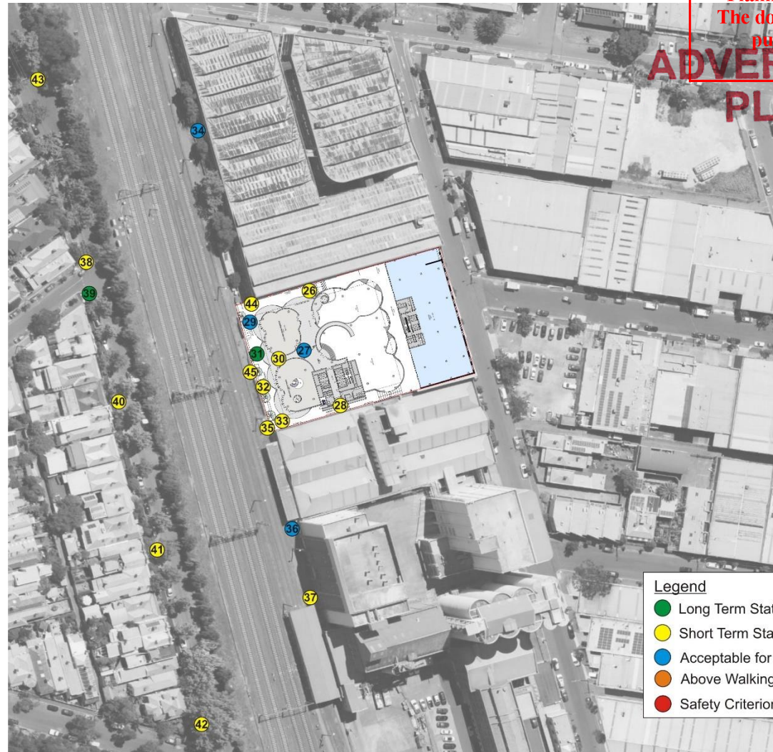
Figure 7a - Summary of wind conditions at Ground Level and West Side Test Locations for the Proposed Young Husband Stage 2 development for the Proposed Configuration for 360° of wind direction
