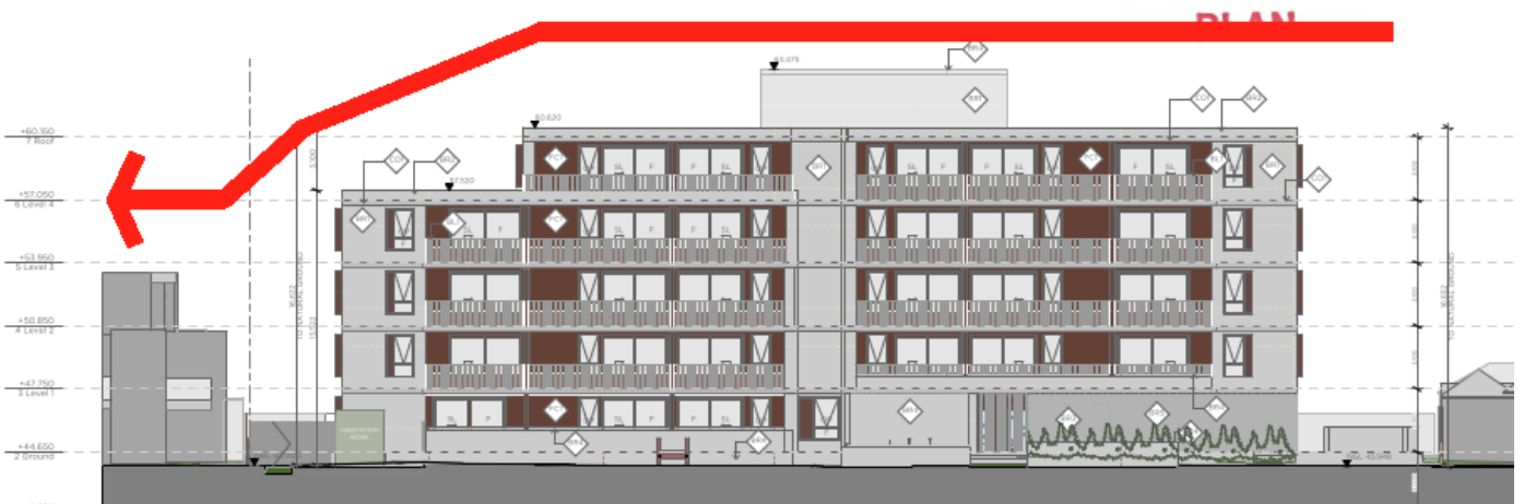
Figure 6 – Diagram of streetscape elevation showing the transition of height from 5 storeys to down the 3-storey building at 45 Rosstown Road
