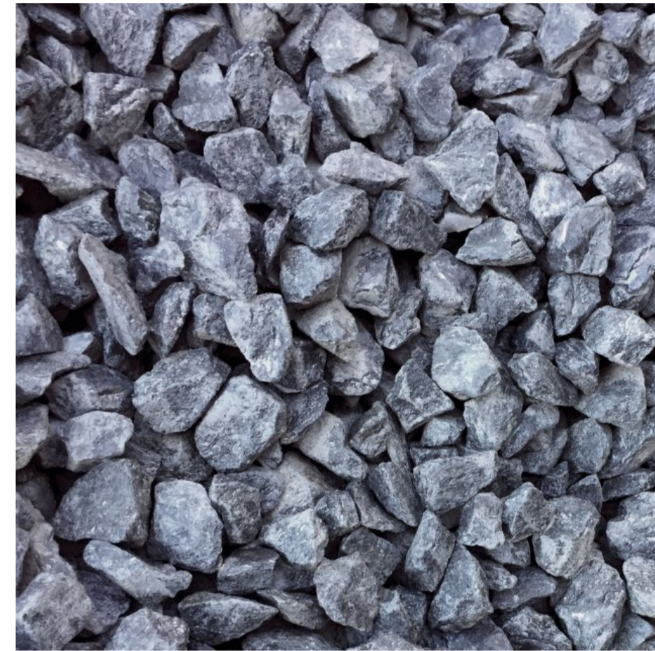
Blue metal - drainage aggregate
