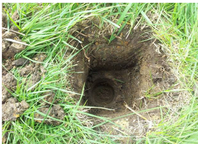
Photo 4: Typical Borehole through Fill.
