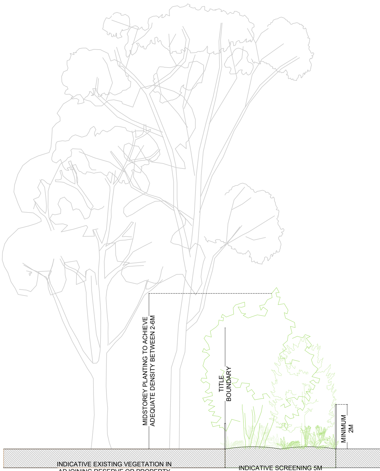
4 INDICATIVE 5M VEGETATION INFILL SCREENING 508-PL SECTION 1:100
