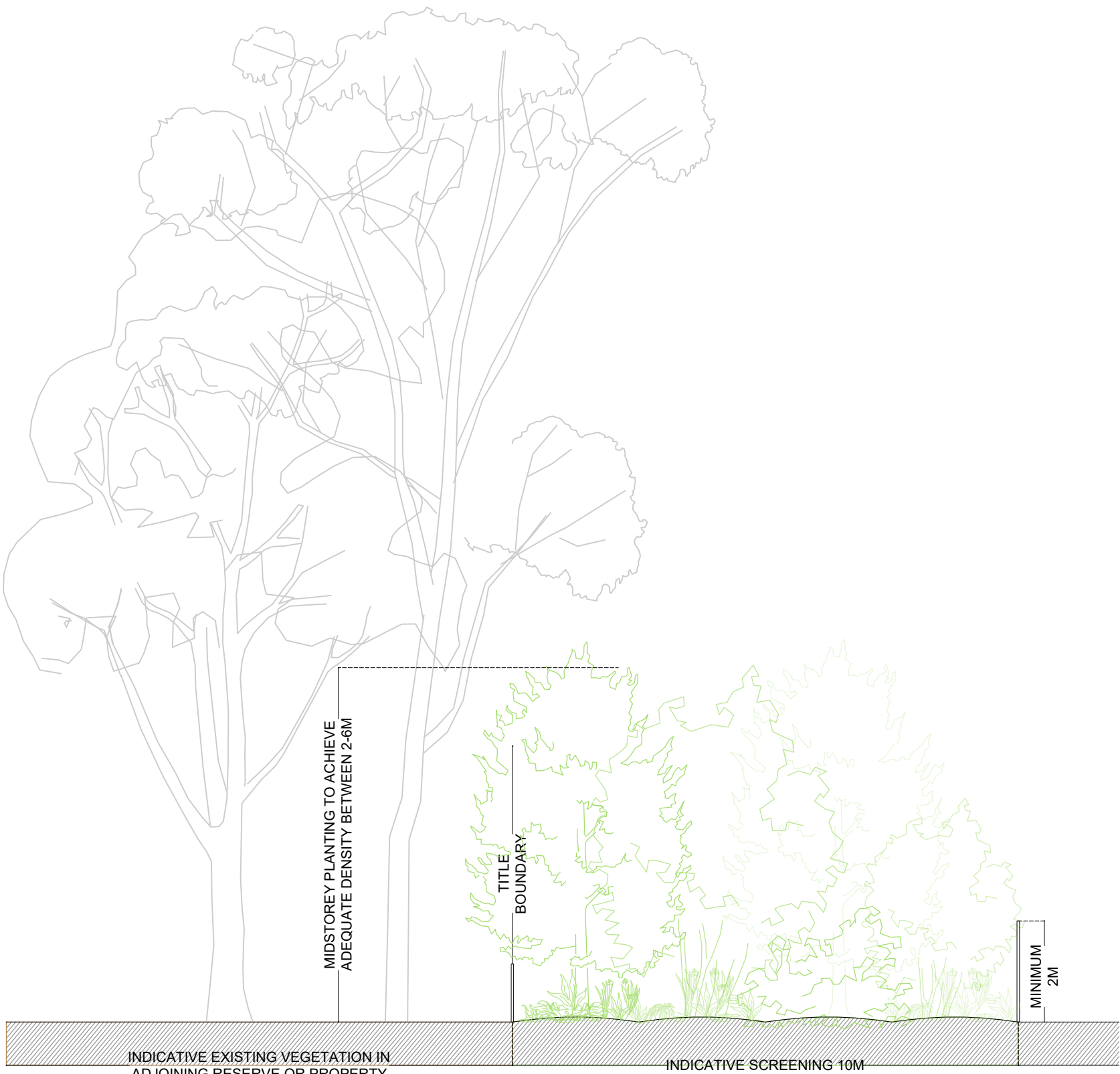
3 INDICATIVE 10M VEGETATION INFILL SCREENING 508-PL SECTION 1:100
