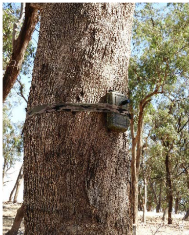
Image 11. Anabat® detector, with microphone attached, mounted to tree
