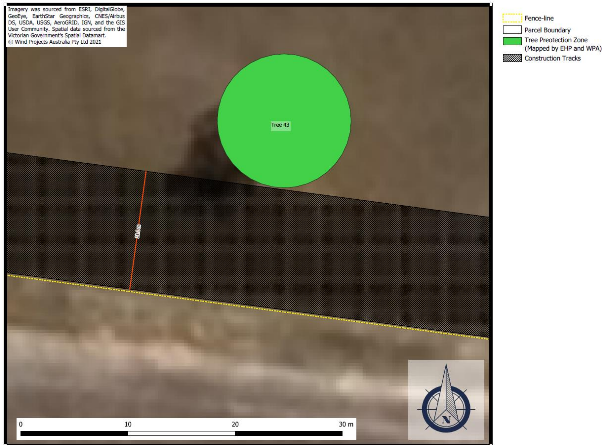
Figure 51: 11.1 m wide construction track passing by Tree 43, as mapped by EHP in their Biodiversity Impact Assessment presented in Appendix 2: Ecological Impact Report. Tree 43 is a Allocasuarina luehmannii with a diameter at breast height of 0.52 m.
