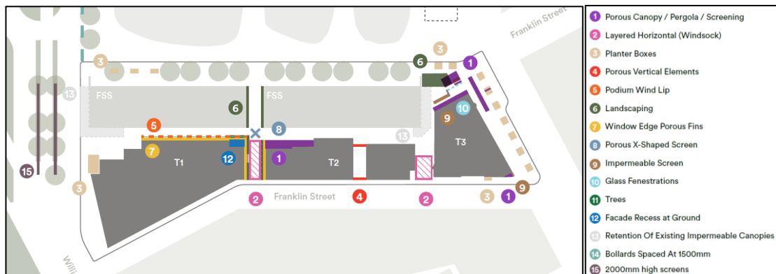
Figure 23: Wind mitigation measures required by the DP
