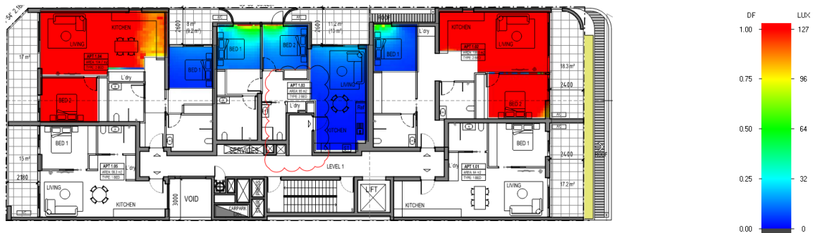
Figure 5 – Scenario B: Daylight map L1 of 17 Taylor Street, Moorabbin modelled with building of same and setback as 17 Taylor St
