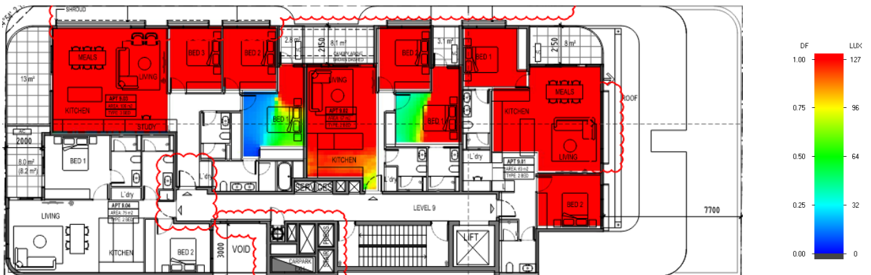
Figure 5 – Scenario B: Daylight map L9 of 17 Taylor Street, Moorabbin modelled with building of same height and setbacks as 17 Taylor St.
