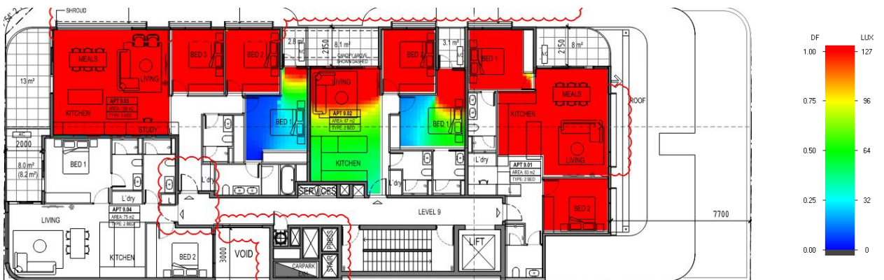
Figure 6 – Scenario C: Daylight map L9 of 17 Taylor Street, Moorabbin modelled with proposed development.
