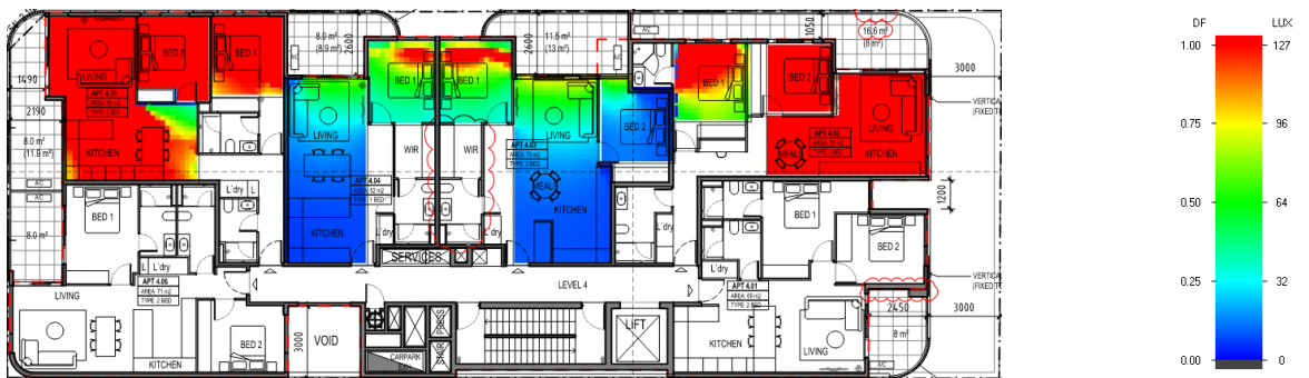
Figure 6 – Scenario C: Daylight map L4 of 17 Taylor Street, Moorabbin modelled with proposed development.
