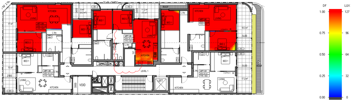
Figure 4 – Scenario A: Daylight map L1 of 17 Taylor Street, Moorabbin modelled with existing developments adjacent.
