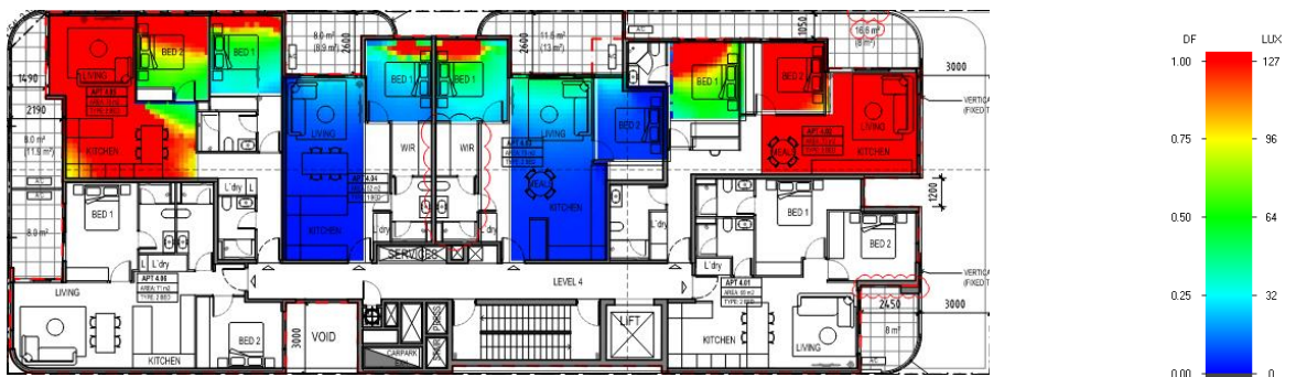
Figure 5 – Scenario B: Daylight map L4 of 17 Taylor Street, Moorabbin modelled with building of same height and setbacks as 17 Taylor St.
