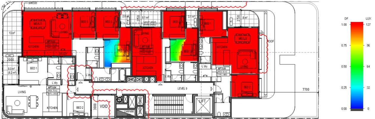
Figure 4 – Scenario A: Daylight map L9 of 17 Taylor Street, Moorabbin modelled with the existing buildings adjacent.
