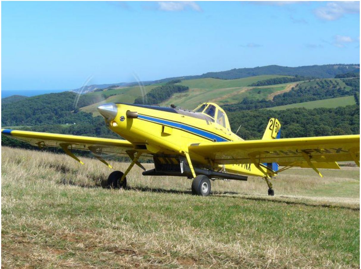
Figure 3 – An Air Tractor AT 502B taxiing. Note the grass surface and its slope. The aircraft is configured for spreading.
