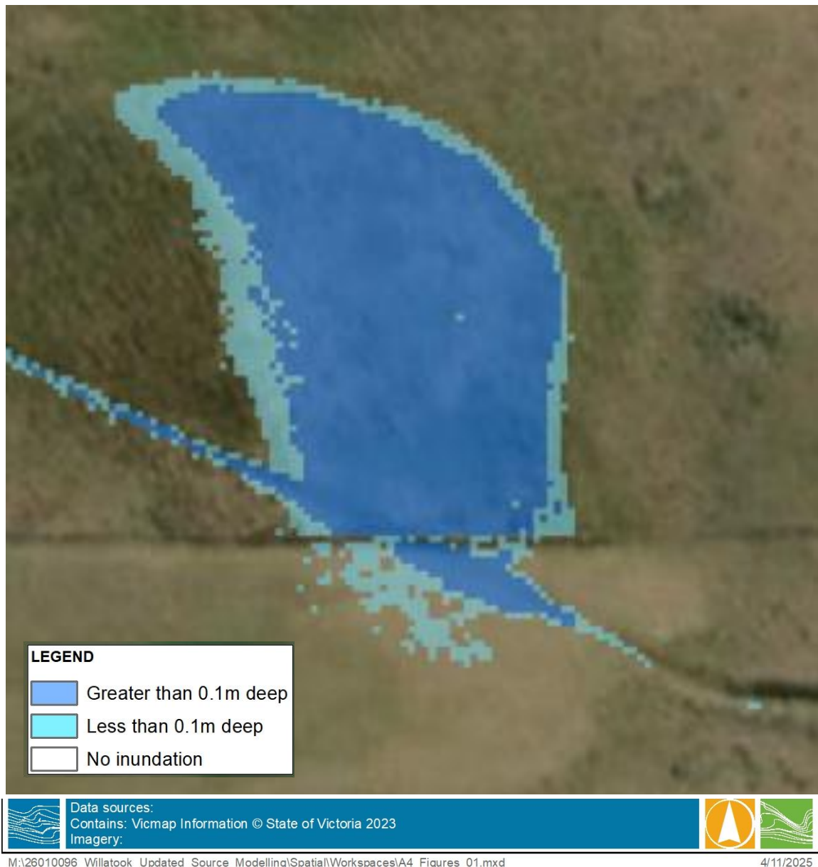
Figure 4-10 Wetland 25626 subsection Potential water extents at maximum water depth and area deeper than 0.1m
