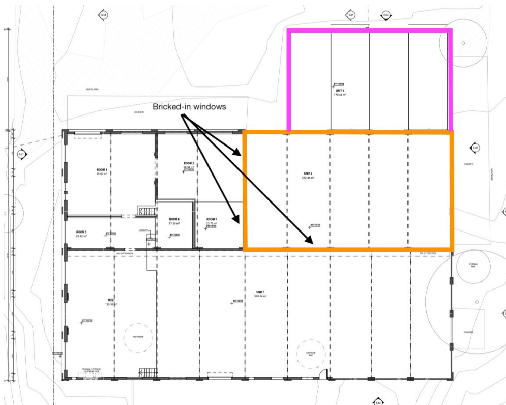
The rear section of the west bay outlined in orange is a later stage of the c.1941 factory, evidenced by bricked up windows in the walls as indicated. The section outlined in purple is a post-World War II addition.
