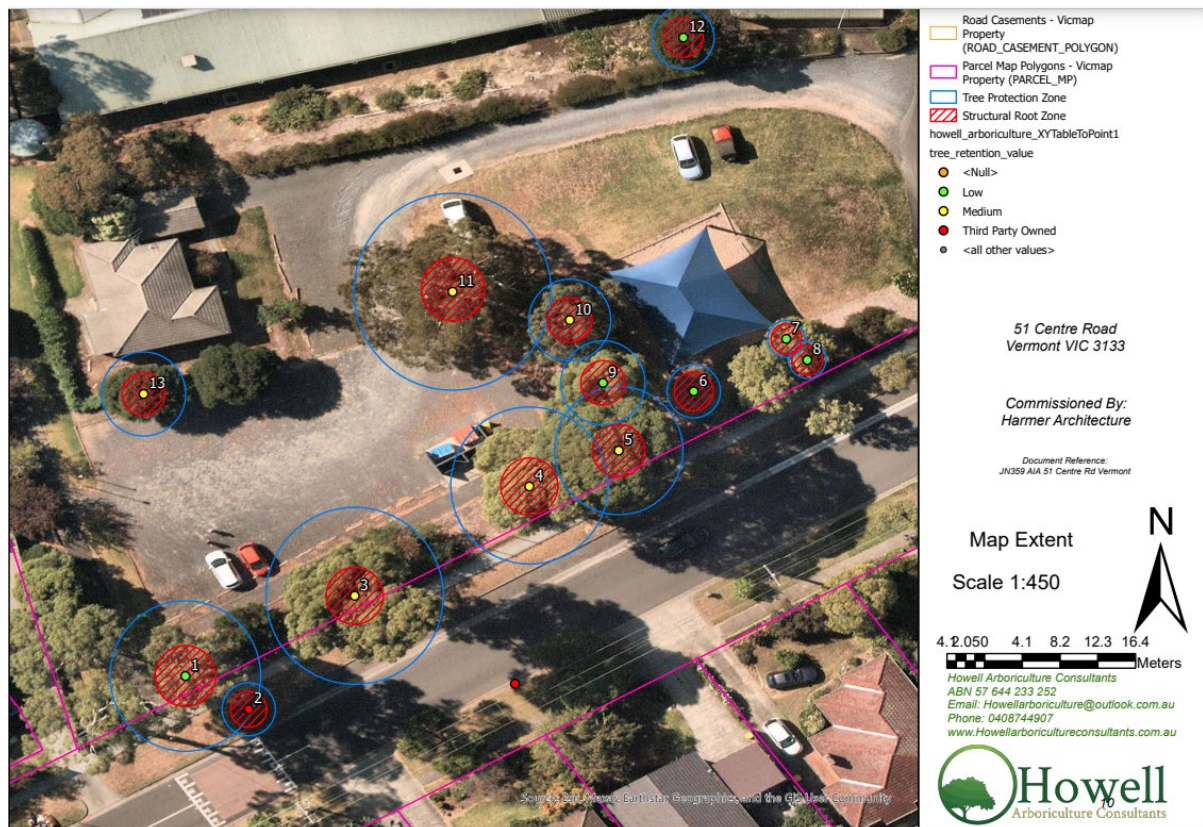
Figure 4: tree structural root zones nominated (source: arborist report)
