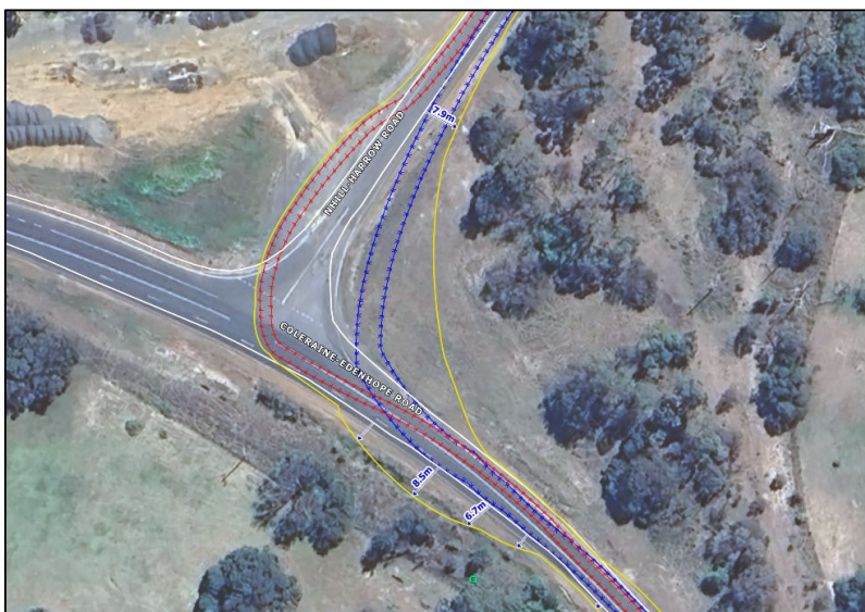
Figure 1. Project set-up included importing transportation shp files (red=front wheel, blue=rear wheel, yellow=swept path, white = existing carriageway). Distances between existing carriageway and swept path (blue arrows) were determined at selected locations to assist with ground truthing.
