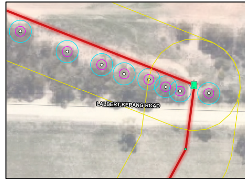
Figure 7. Section of external transmission line crossing Lalbert-Kerang Rd. The proposed route is of low risk to surrounding trees in terms of projected TPZs and likely boring pit locations.
