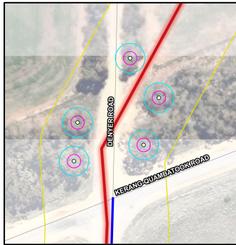
Figure 6. Section of external transmission line crossing Kerang-Quambatook Rd. The proposed route avoids TPZ incursion and is of low risk to existing trees.
