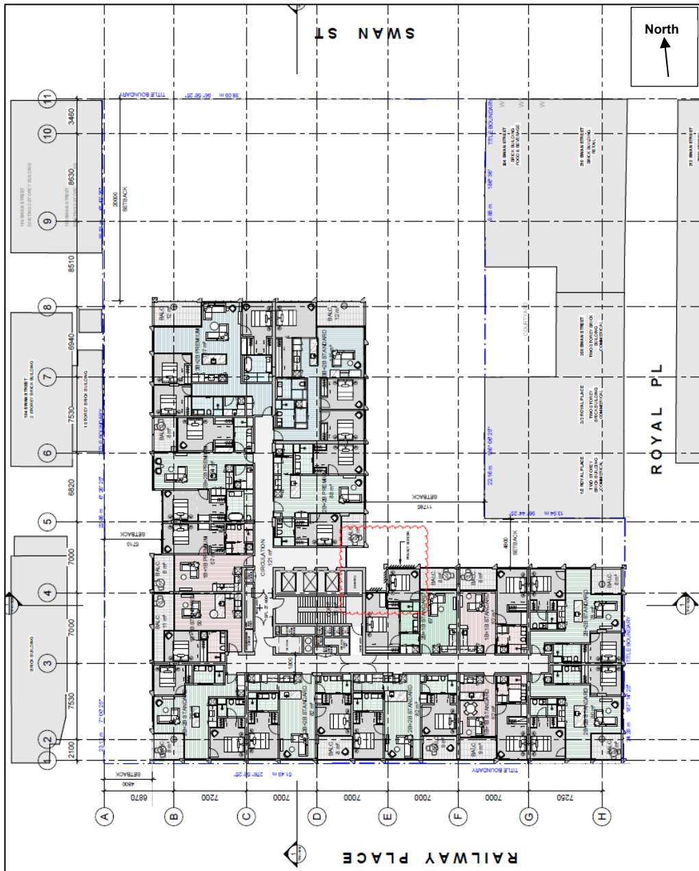
Figure 7: Level 5 floor plan (floor plans for Levels 6 to 10 are the same) of the proposed 188-202 Swan Street Development.
