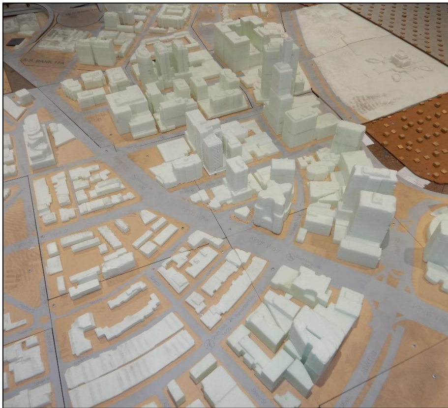
Figure 2a - View from the south of the 1/400 scale model of the proposed 60-70 Park Street development in the wind tunnel.
