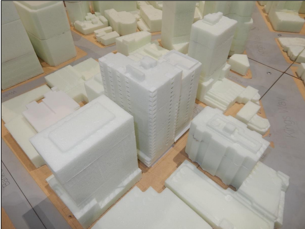
Figure 2d - Close-up view from the north-west of the 1/400 scale model of the proposed 60-70 Park Street development in the wind tunnel.
