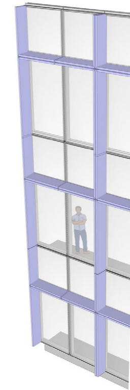
Profiled fin / sunshade - vertical & horizontal (Image above)
