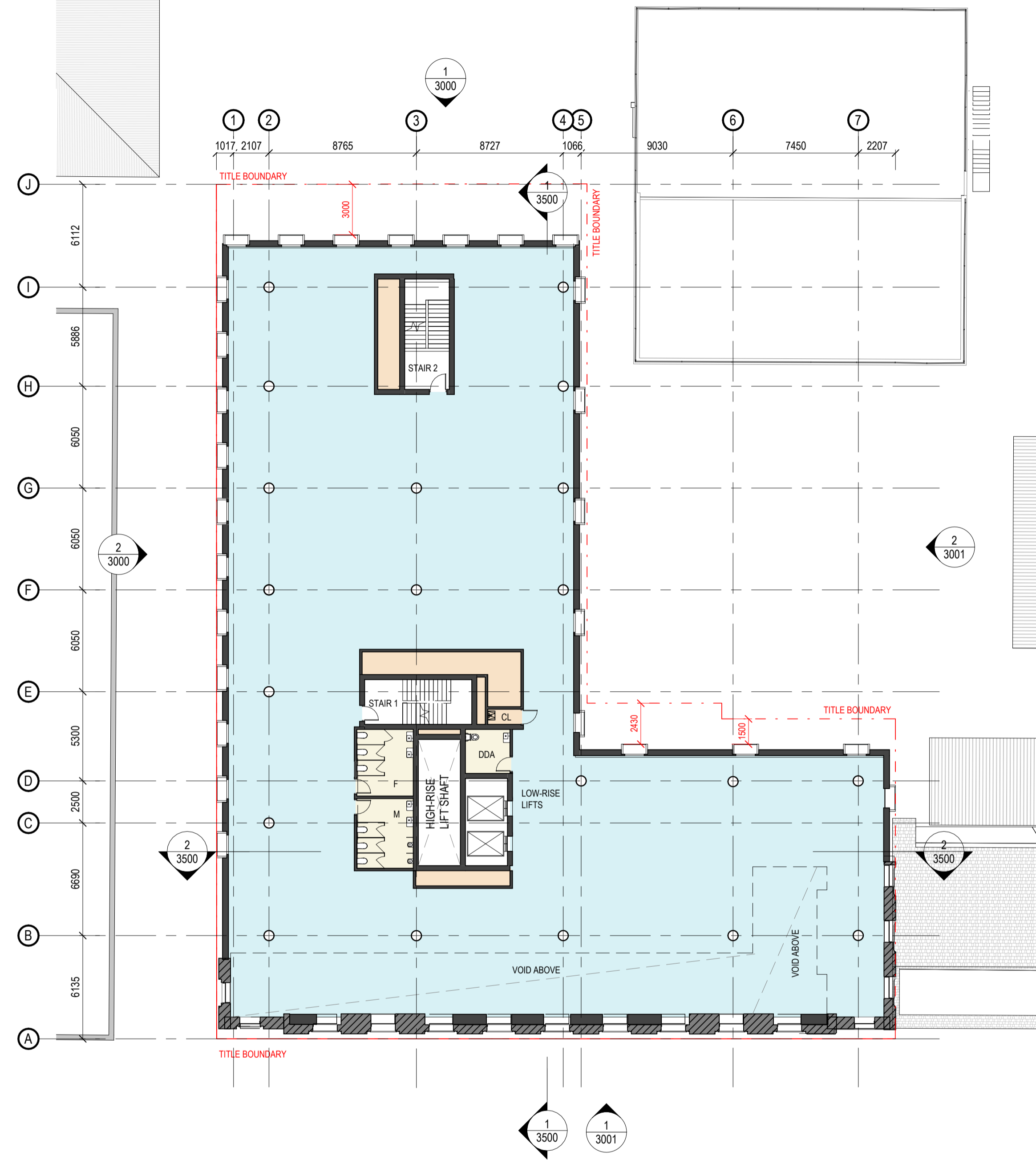
1 FLOOR PLAN - LEVEL L04 Scale 1 : 200
