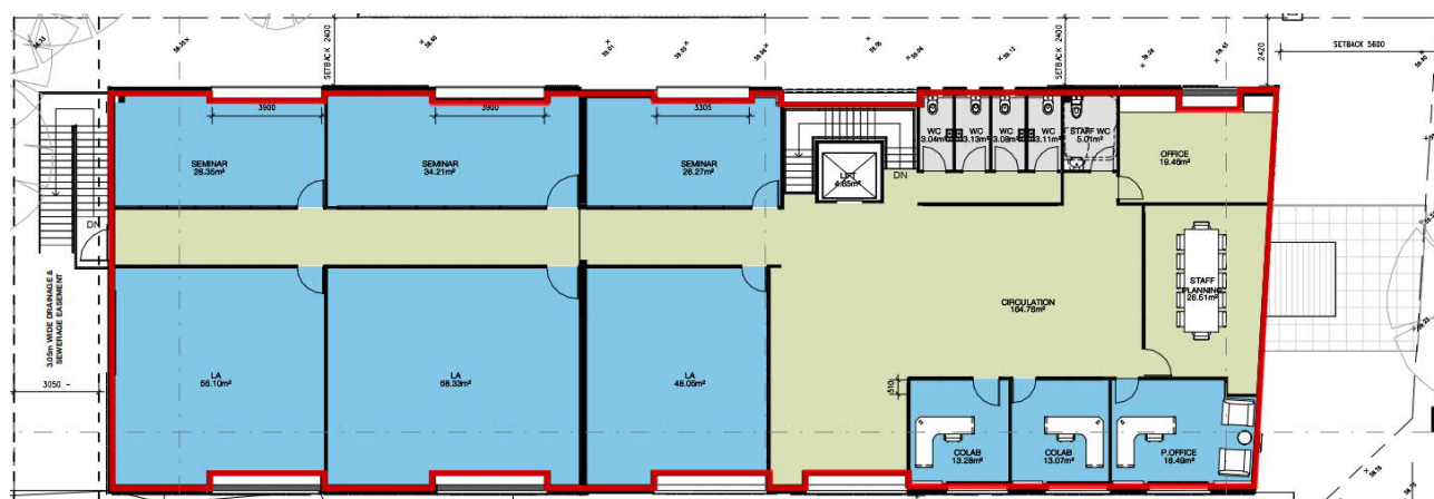
Figure 14: Level 1 walls required to achieve a total system R-Value of R1.40
