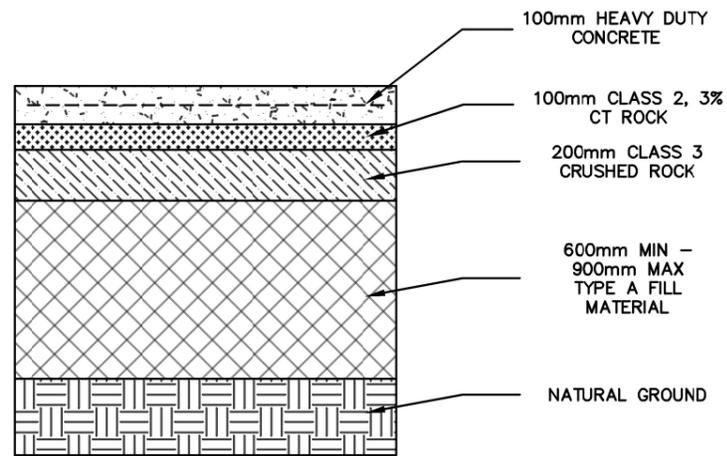
TYPICAL STRUCTURAL SLAB DETAIL:
