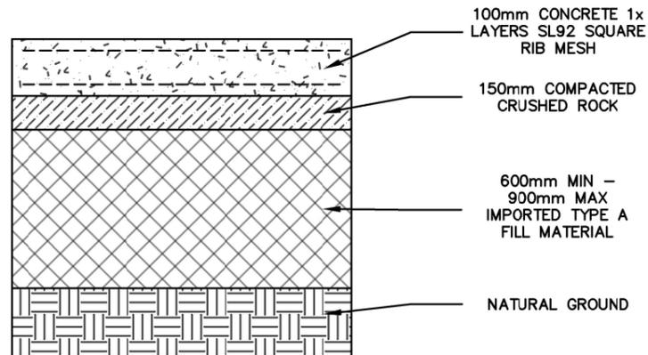
TYPICAL SLAB DETAIL AROUND TANKS AND EQUIPMENT:
