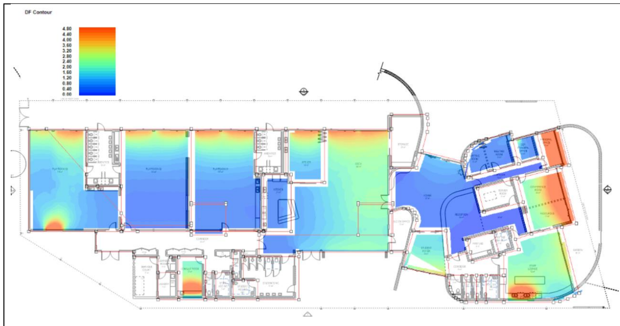
Figure 1: Admin and ELC Building Daylight Modelling Contours
