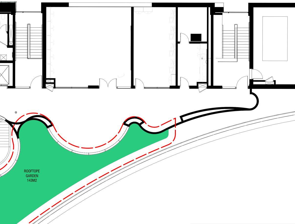
GB2 - 500mm soil depth fully tanked and drained irrigated garden bed on structure
