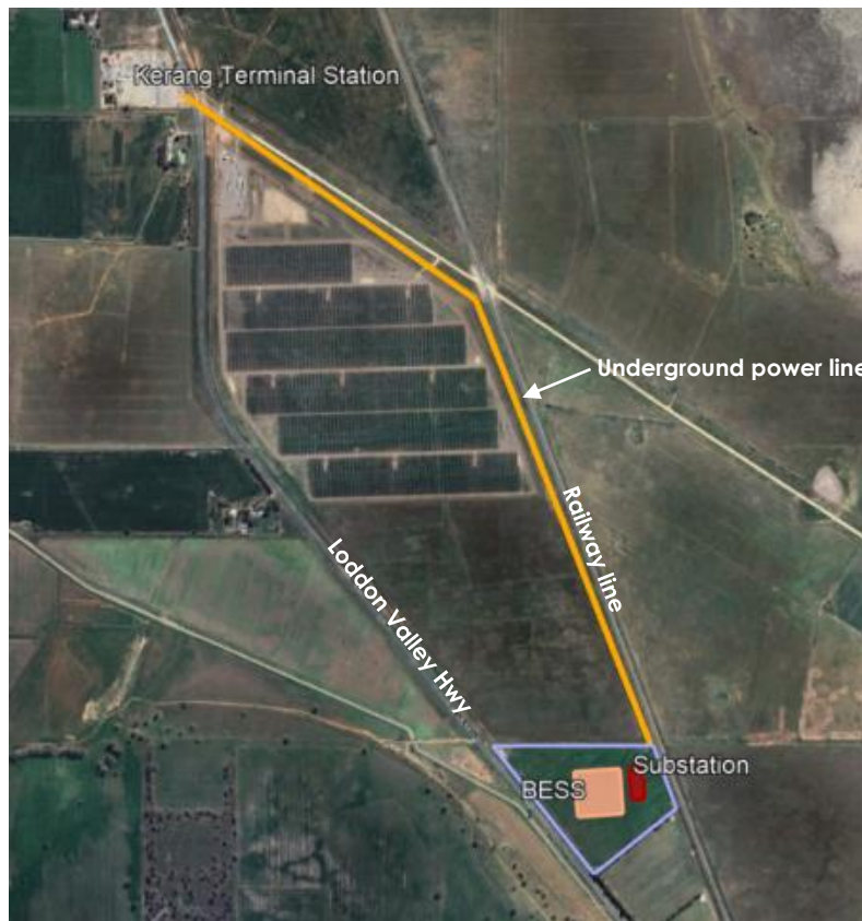
Figure 4 – Alignment of proposed connecting underground transmission line route (Source: Google Earth).
