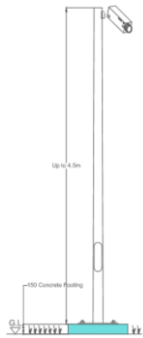
Figure 13 – Typical post mounted security camera.
