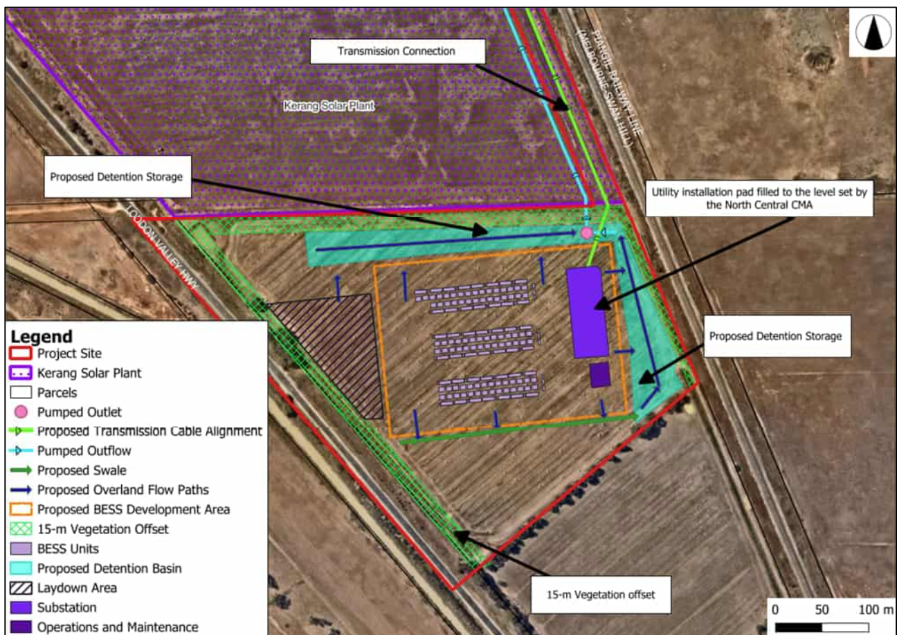
Figure 11: Stormwater Management Overview Plan – Typical Conditions
