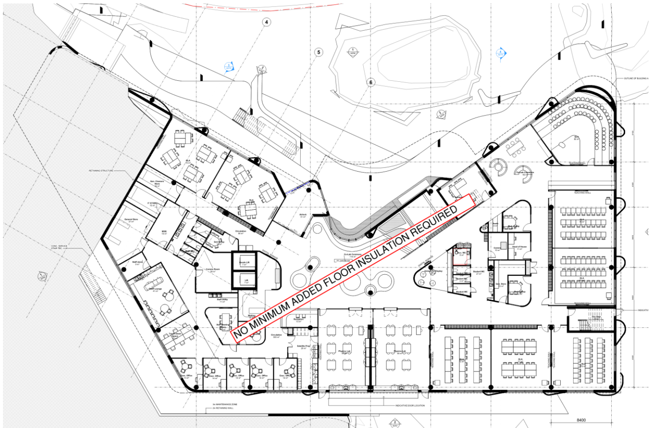
Figure 34: Floor Insulation Requirements – Lower Ground Floor
