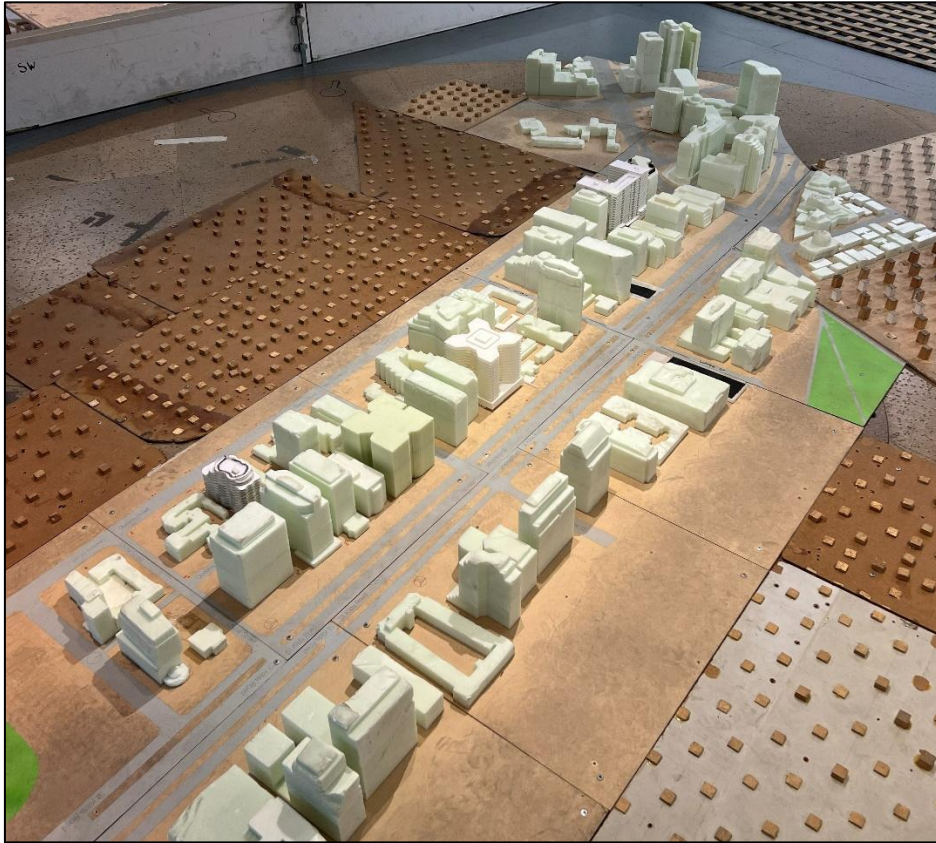
Figure 2b - View from the south-east of the 1/400 scale model of the proposed 464 St Kilda Road development in the wind tunnel.
