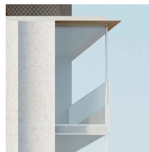
CODE: GLZ-03 DESCRIPTION: FACADE GLAZING MATERIAL: SINGLE GLAZED WIND SCREEN IN POWDERCOATED ALUMINIUM FRAME FINISH: CLEAR GLASS / POWDERCOATED ALUMINIUM COLOUR: GULL MATT POWDERCOAT FRAME
