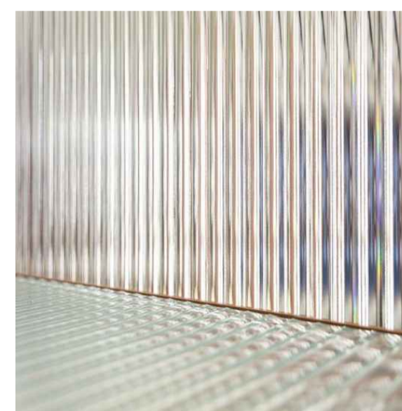
CODE: GLZ-04 DESCRIPTION: FACADE GLAZING MATERIAL: DOUBLE GLAZED UNIT WITH LOW-IRON CLEAR FLUTED GLASS IN POWDERCOATED ALUMINIUM FRAME FINISH: LOW-IRON CLEAR GLASS / POWDERCOATED ALUMINIUM COLOUR: GULL GREY MATT POWDERCOAT FRAME
