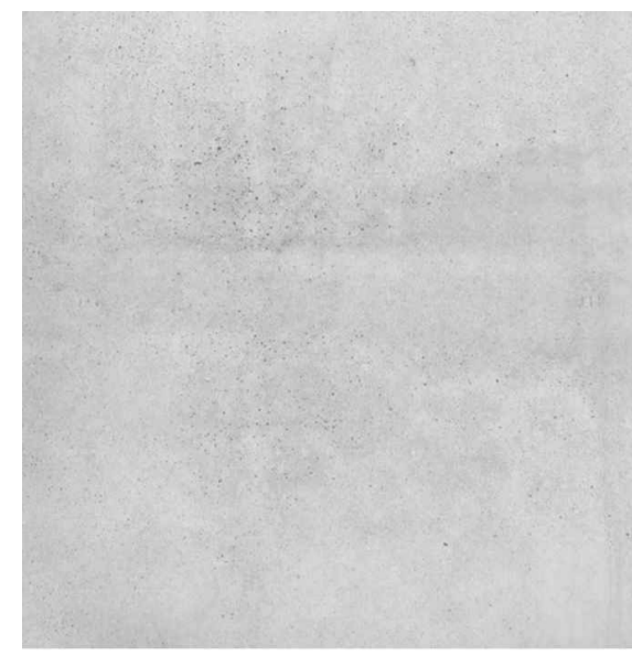
CODE: CFC-01 DESCRIPTION: EXTERNAL CLADDING MATERIAL: COMPRESSED FIBRE CEMENT CLADDING FINISH: RAW/NATURAL FINISH COLOUR: FULL-DEPTH THROUGH COLOUR IN OFF-WHITE TO MATCH C-01 COLOUR
