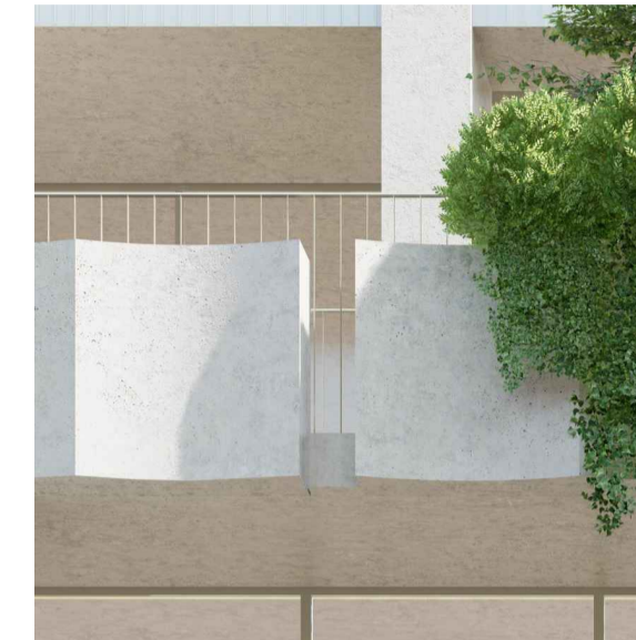
CODE: BAL-02 DESCRIPTION: BALUSTRADE MATERIAL: GLASS-FIBRE REINFORCED PLANTER BOXES WITH SCALLOPED PROFILE. METAL BALUSTRADE ON INSIDE FACE WITH NOM. 50x10 VERTICALS & TOP RAIL FINISH: PLANTER BOXES: OFF-FORM FINISH CLASS 1, BALUSTRADE: GALVANISED COLOUR: WHITE BRIGHTONLITE CEMENT (INTEGRAL OXIDE COLOUR) TO MATCH C-01
