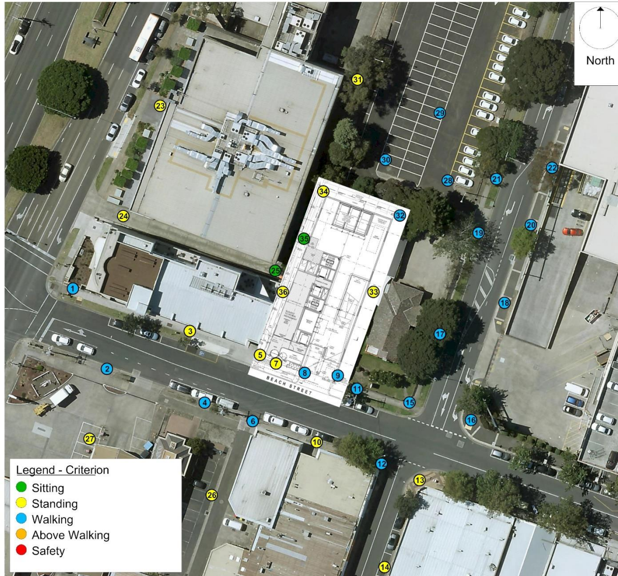
Figure 6a - Summary of wind conditions for the proposed 11 Beach Street, Frankston Development for the Proposed Configuration for 360° of wind direction.
