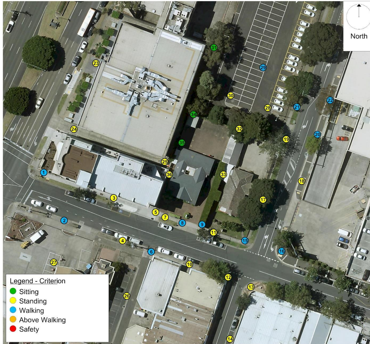
Figure 5 - Summary of wind conditions for the proposed 11 Beach Street, Frankston Development for the Existing Configuration for 360° of wind direction.
