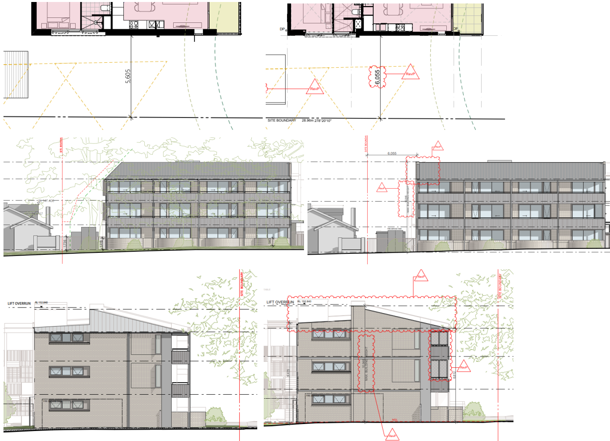
Figure 8. Decision plans (left) and current proposed amendment (right) showing the increase in the southern setback and adjustments to roof form at the southern edge of the east wing of the apartment building.
