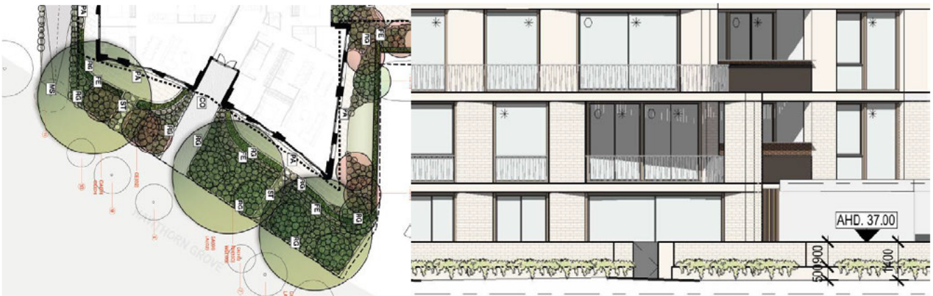
Figure 40 – Excerpt from landscape plan of generous front landscaping area and canopy tree planting in Hawthorn Grove (left) and elevation of Hawthorn Grove fencing, demonstrating all front landscaping is contained behind low height retaining walls and forward of higher private courtyard fencing.
