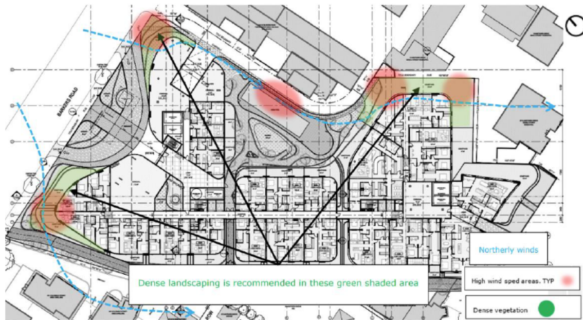
Figure 36 – Excerpt from Wind Impact Assessment demonstrating main areas of concern within and surrounding the development for windspeeds and recommended location for mitigation measures to counteract these.
