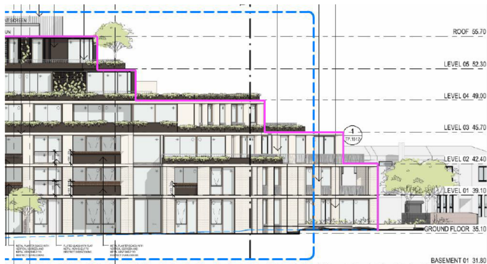
Figure 31 – Excerpt from the western elevation, with emphasis in pink of the progressive, stepped heights and setbacks of the building down to the double storey street wall to Hawthorn Grove.
