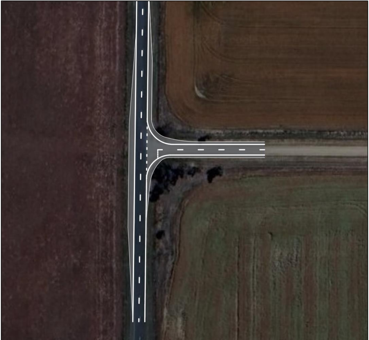
Figure 8-17: Roslynmead Road / Chrystal Road intersection upgrade concept sketch
