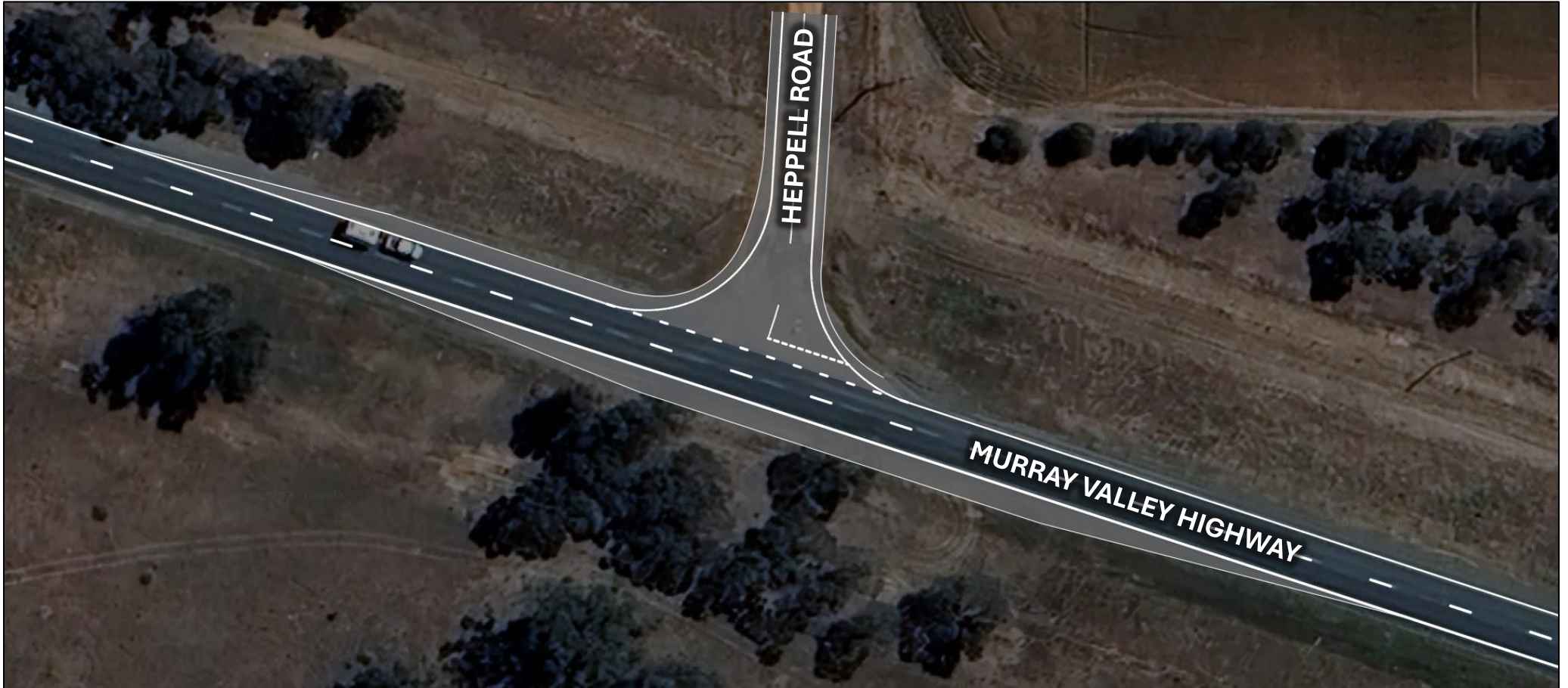
Murray Valley Highway / Heppell Road intersection upgrade concept sketch (BAR / BAL layout)
