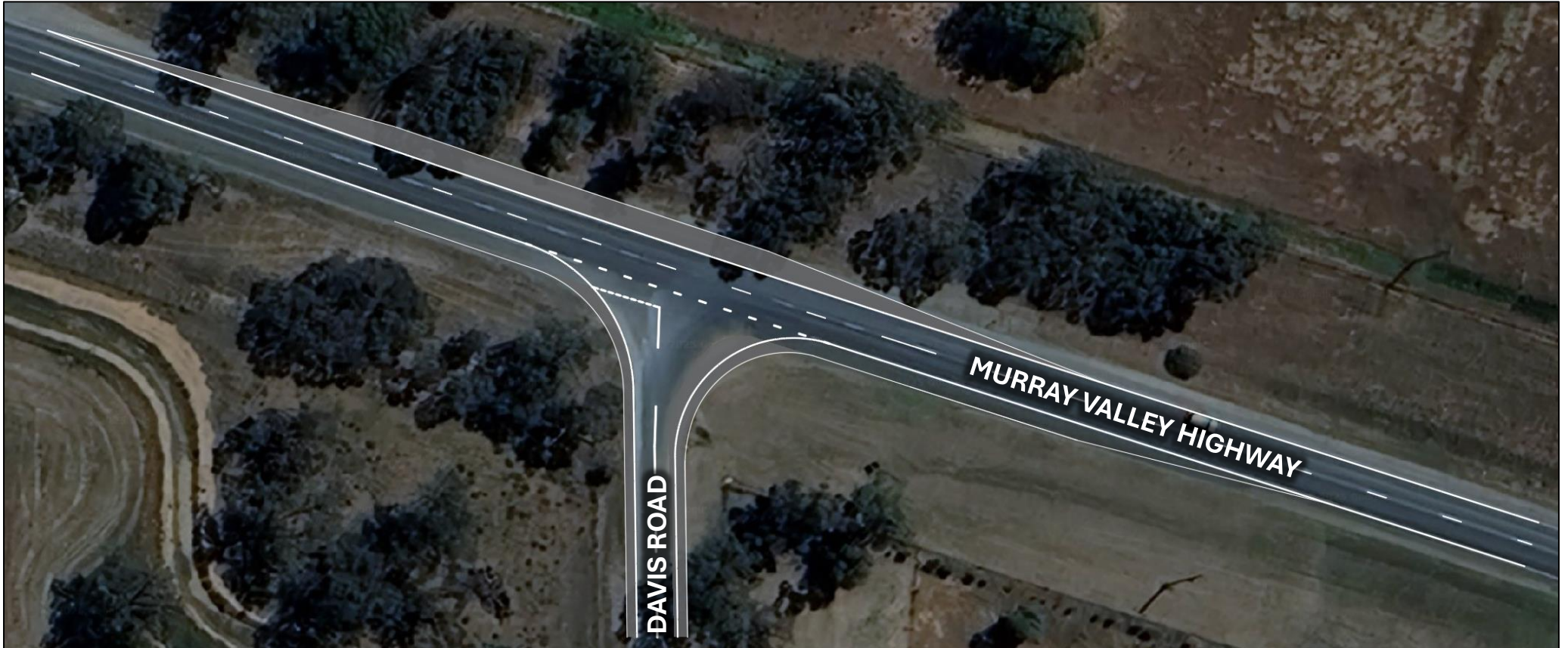
Murray Valley Highway / Davis Road intersection upgrade concept sketch (BAR / BAL layout)
