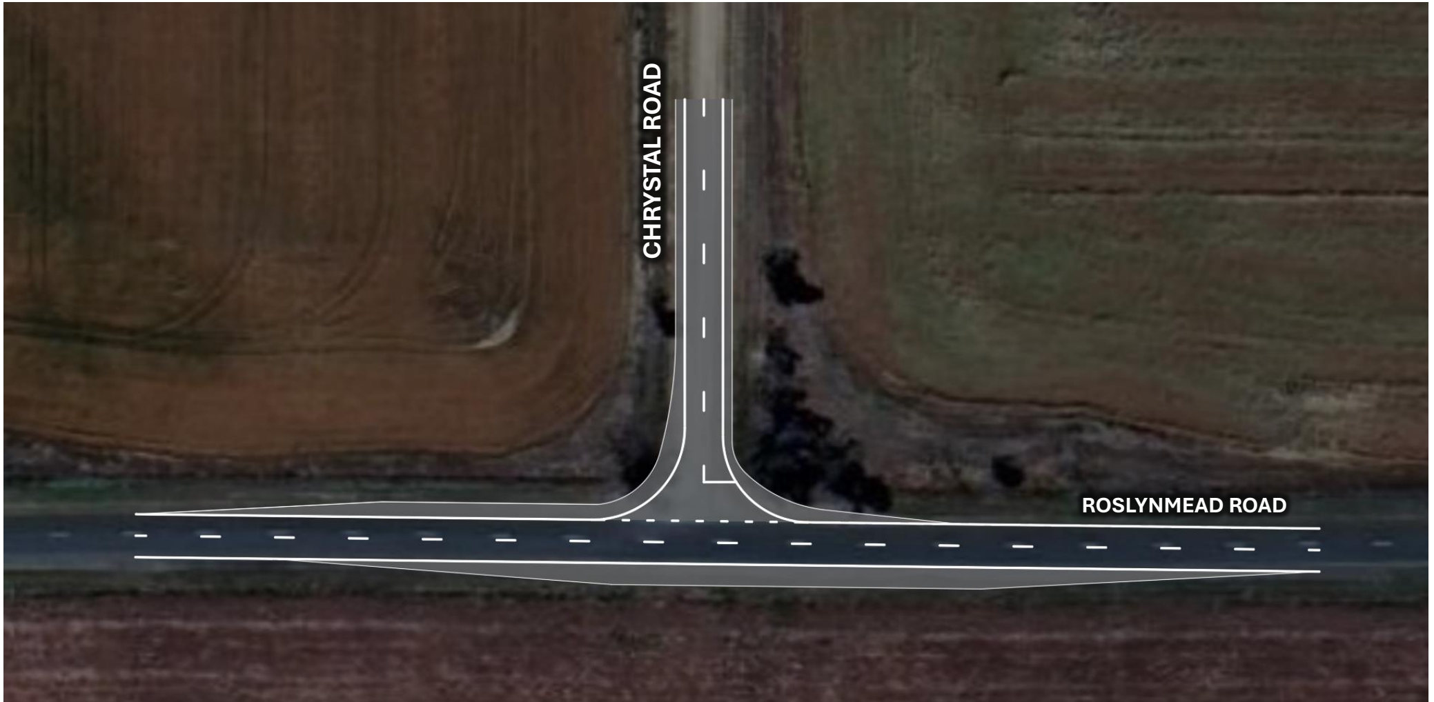
Roslynmead Road / Chrystal Road intersection upgrade concept sketch (BAR / BAL layout)
