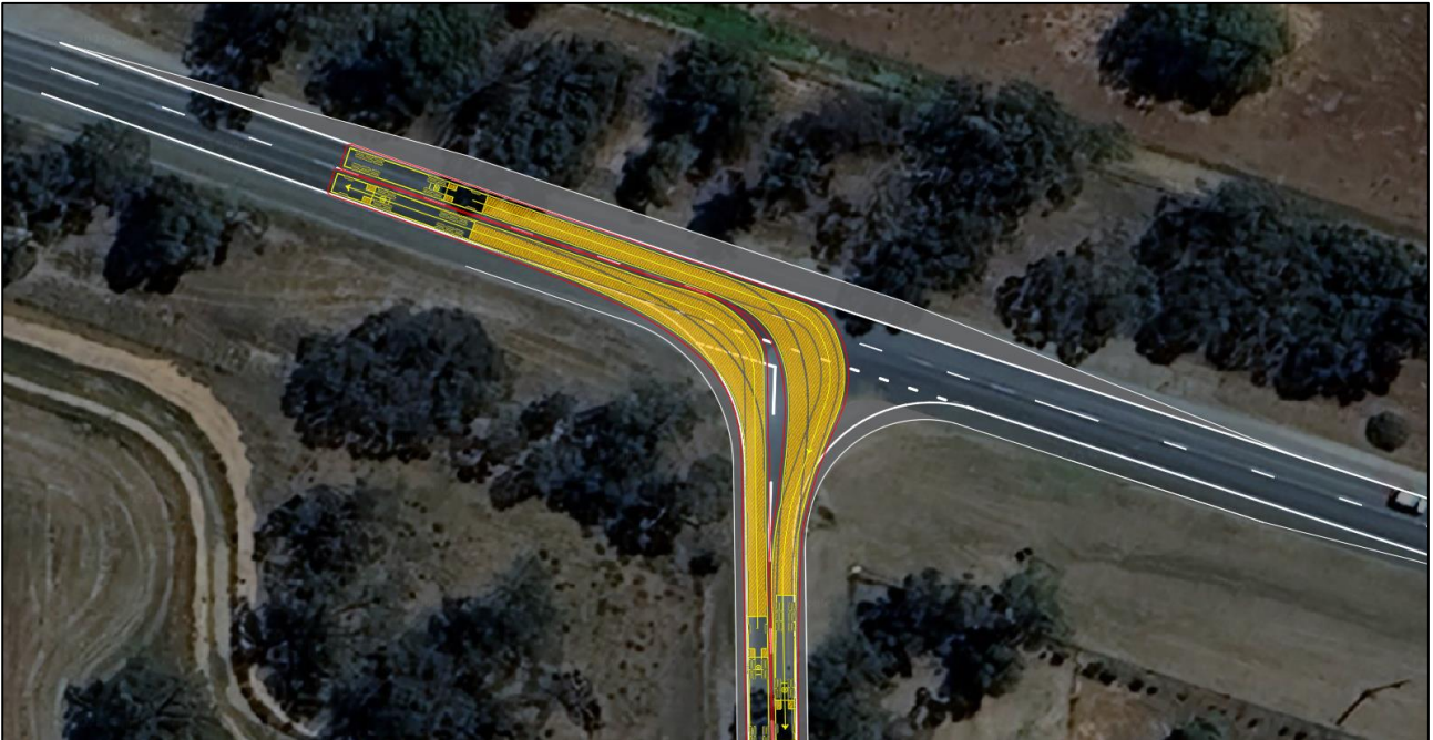
Figure 8-9: Murray Valley Highway / Davis Road – 19m AV turn path – Right In / Left Out
