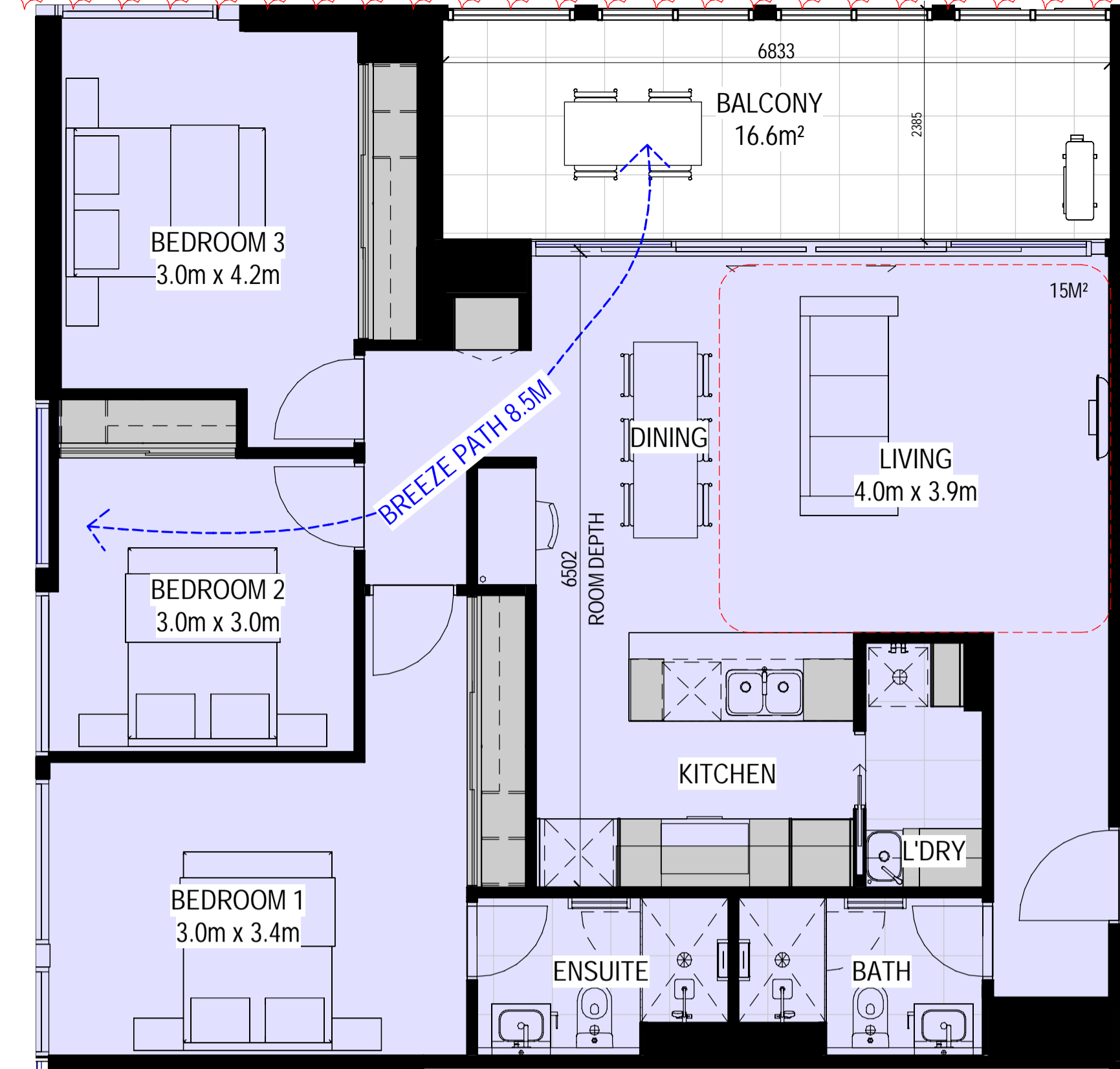
TYPE P 3 BEDROOM APARTMENT INTERNAL AREA - 104M 2 BALCONY - 16.6M 2 2 INSTANCES INTERNAL STORAGE - 18.8M 3 OVERALL STORAGE - 23.7M 3
