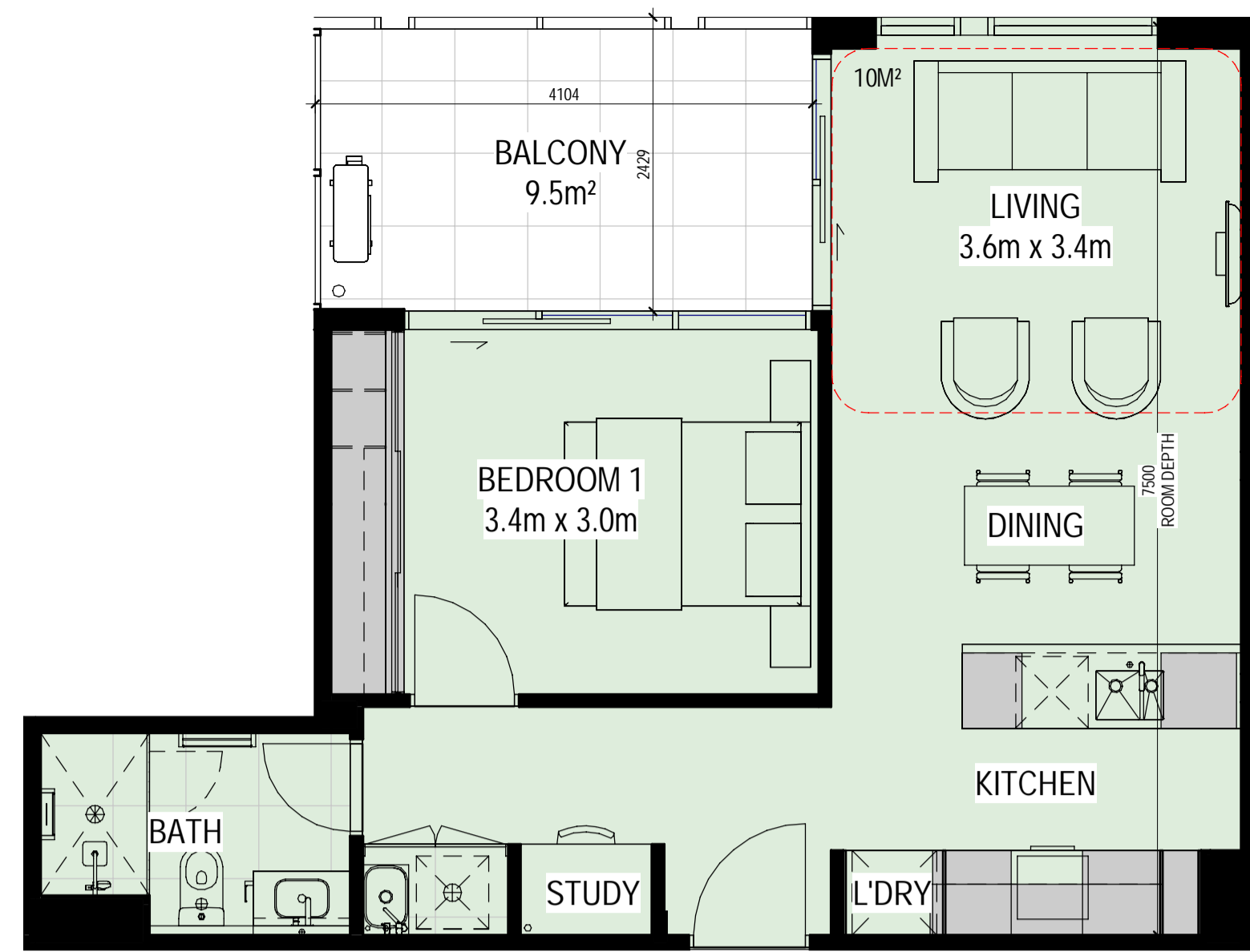
TYPE I 1 BEDROOM APARTMENT INTERNAL AREA - 55M 2 BALCONY - 9.5M 2 11 INSTANCES INTERNAL STORAGE - 7.3M 3 OVERALL STORAGE - 10.7M 3
