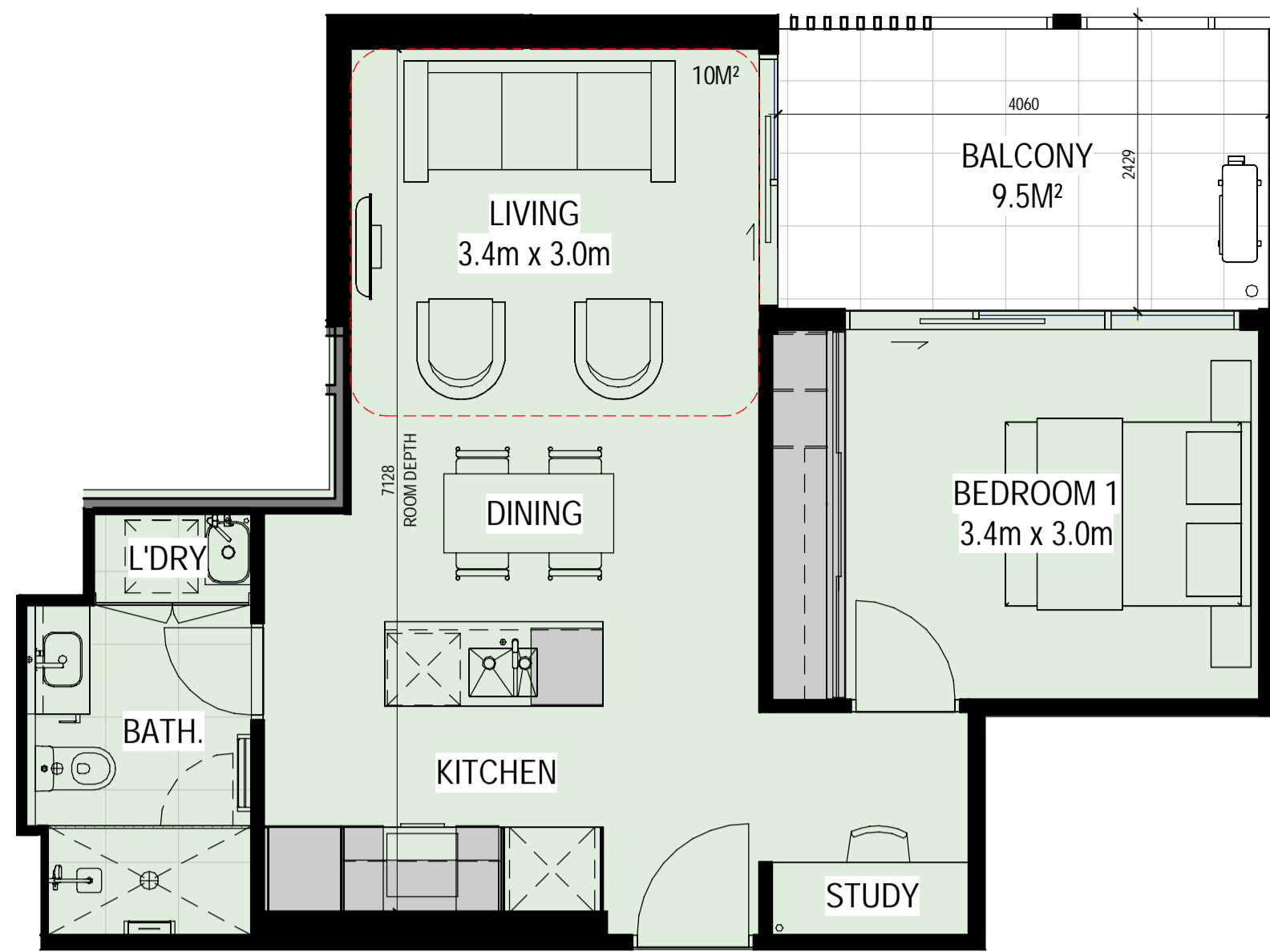
TYPE H 1 BEDROOM APARTMENT INTERNAL AREA - 54M 2 BALCONY - 9.5M 2 11 INSTANCES INTERNAL STORAGE - 7.2M 3 OVERALL STORAGE - 10.0M 3
