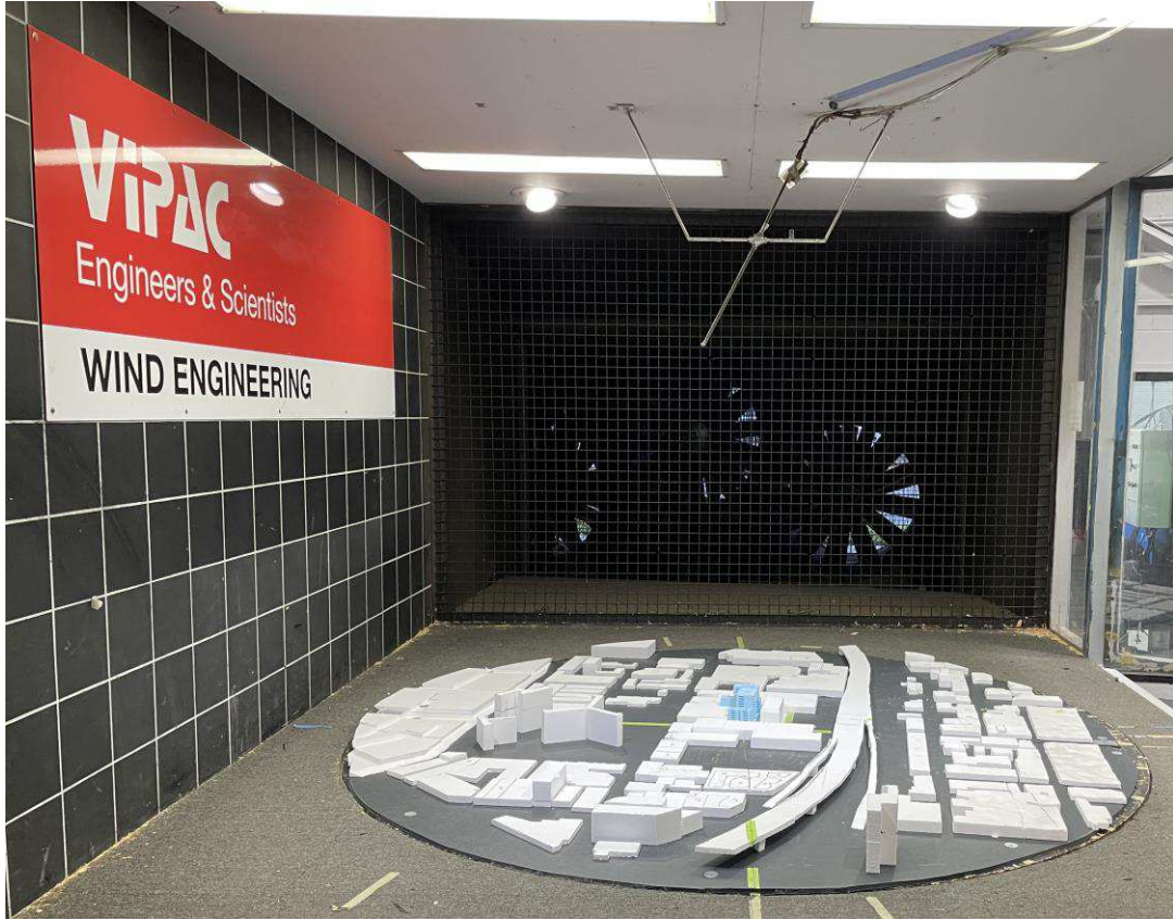
Figure 5: Overall view from north of the 1:400 scale model of the proposed development in the wind tunnel.
