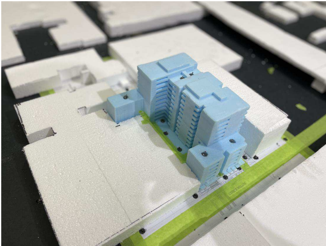
Figure 6: Close up view from the north east of the 1:400 scaled model in the wind tunnel.
