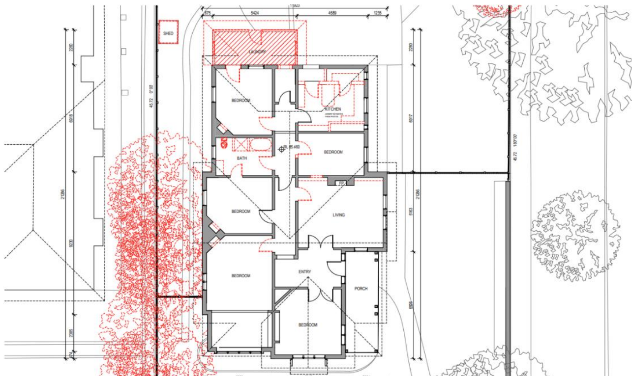
Figure 1 Proposed demolition works at the site
