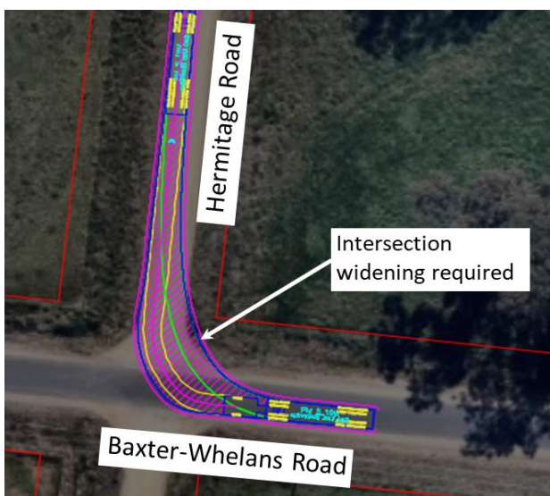
19m Semi-trailer to the site
