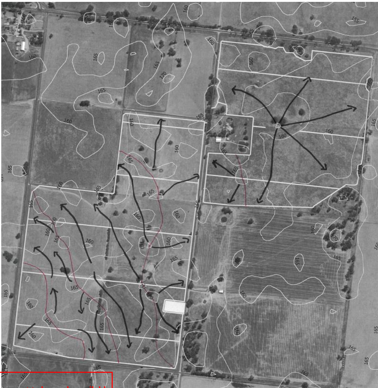
Figure 3-3 Sub-catchments and inferred site runoff directions
