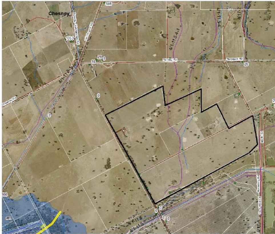
Figure 1: Flood overlay controls (Benalla Planning Scheme) and 1% AEP flood level contour adjacent to the site.
