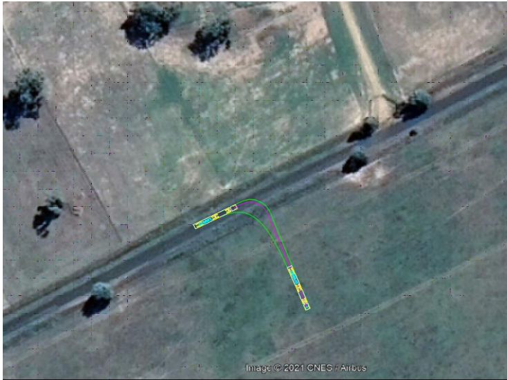
Figure 16 B-Double vehicle swept path on existing geometry of Lake Mokoan Road – Access Point 3
