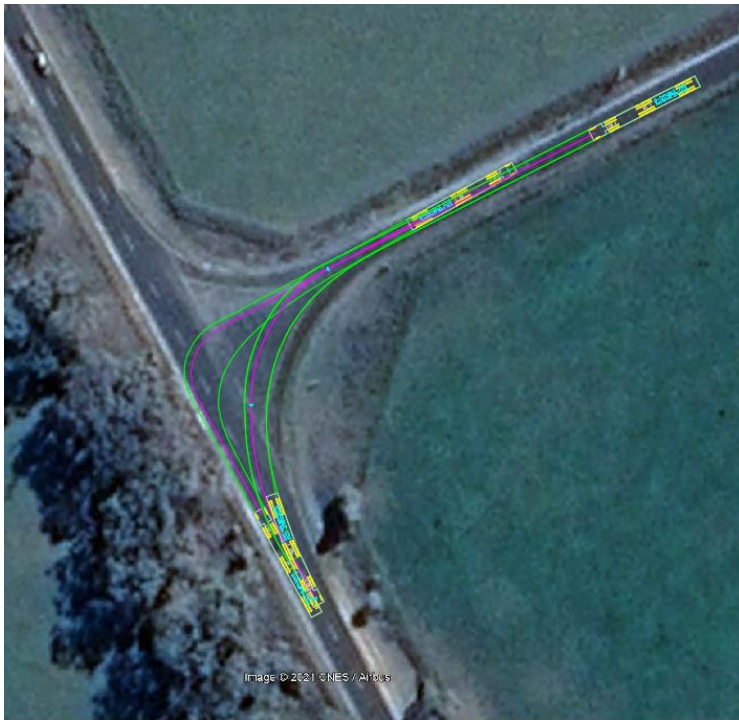
Figure 19 Two-way movement B-Double vehicle swept path on existing geometry of Benalla-Yarrowonga Road and Lake Mokoan Road intersection
