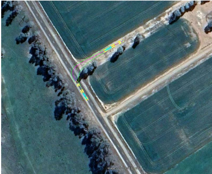
Figure 18 B-Double vehicle swept path analysis on existing geometry of Benalla-Yarrowonga Road (southernmost proposed entry) – Access Point 5
