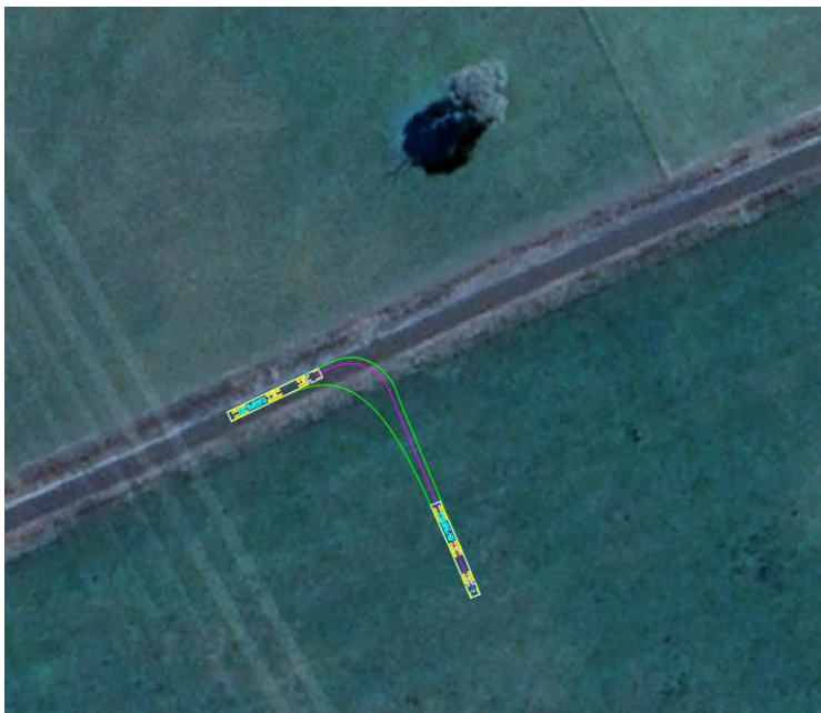
Figure 15 B-Double vehicle swept path on existing geometry of Lake Mokoan Road – Access Point 2
