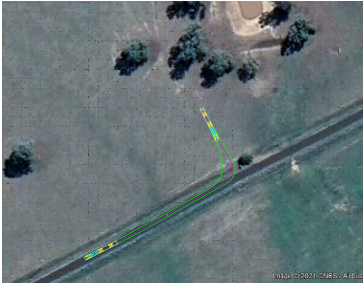
Figure 14 B- Double vehicle swept path on existing geometry of Lake Mokoan Road – Access Point 1
