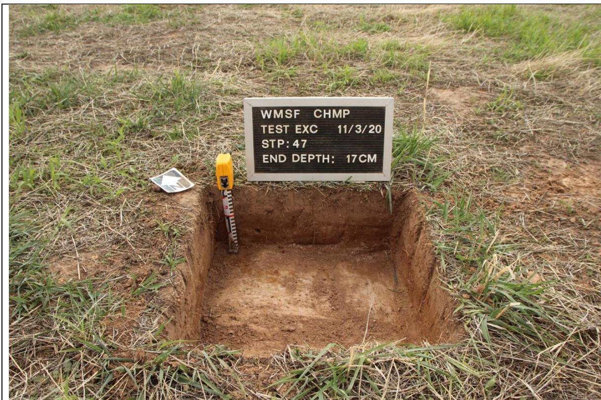
**Plate 9 Texture contrast soil profile in STP TP#47 (Source: AECOM 2020)**
