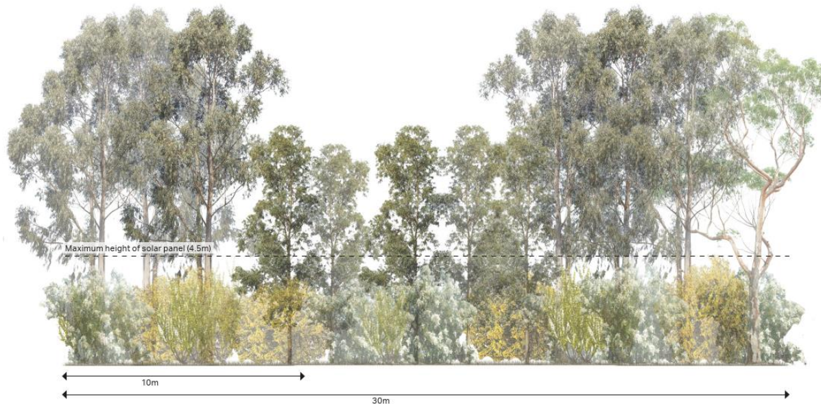
Figure 9 Typical 10m wide screening section - 10 years post installation
