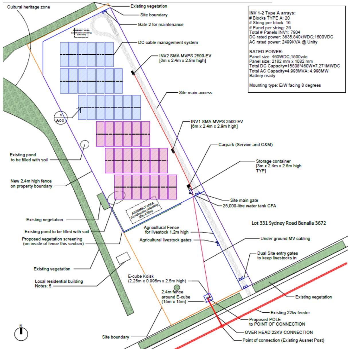
Figure 1: Proposed Layout of Solar Facility
