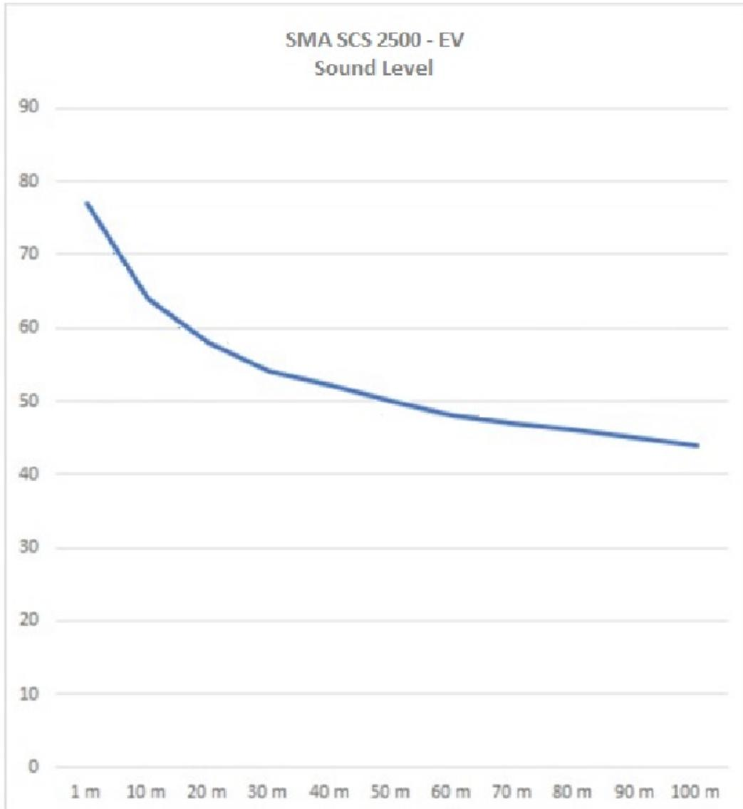
**Figure 2:** Graph of sound power levels over distance
