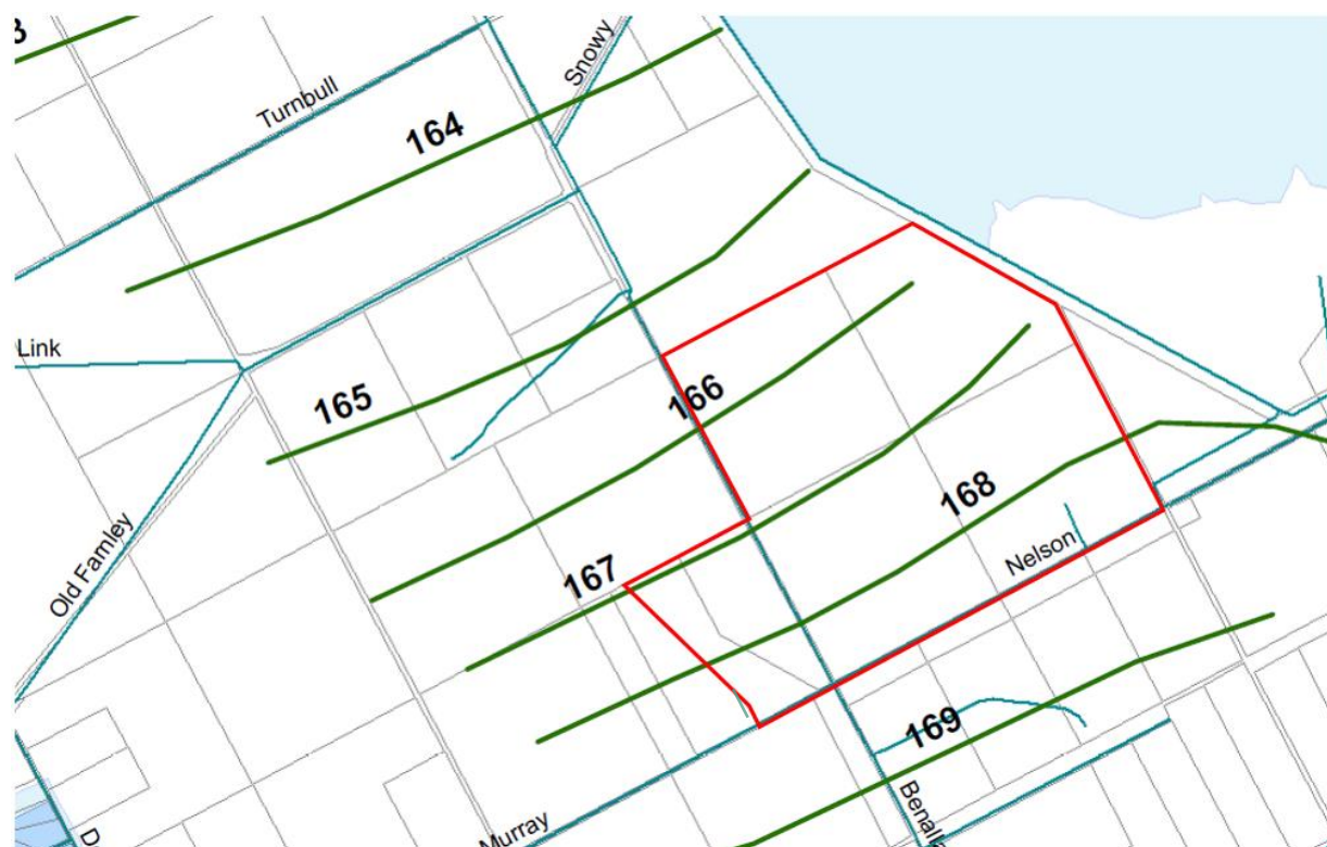
Figure 3 Predicted 1% AEP flood contours shown green (mAHD) across the proposed site outlined in red (Source: GBCMA Flood Atlas)
