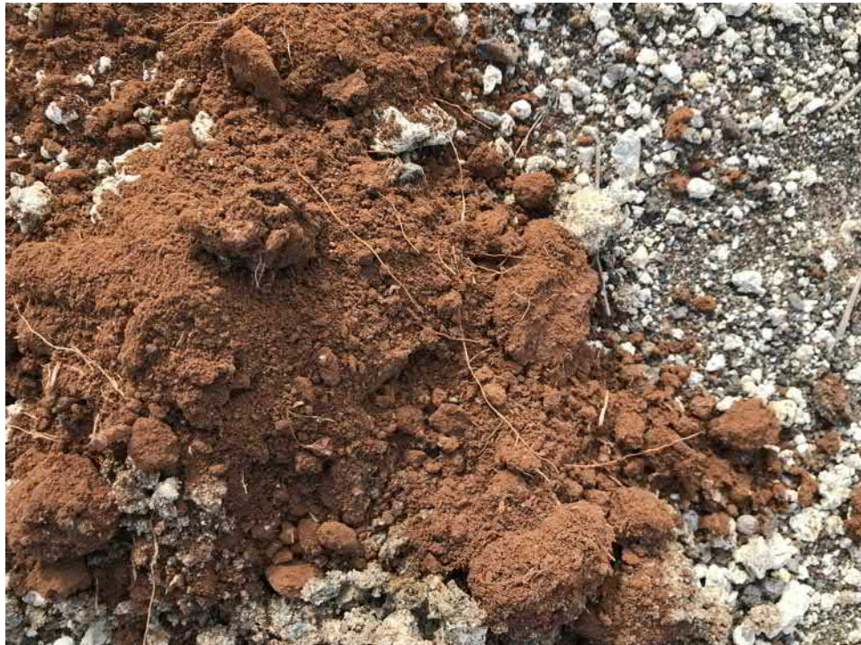
Plate 10: Natural soils underlying fill material at STP07.
