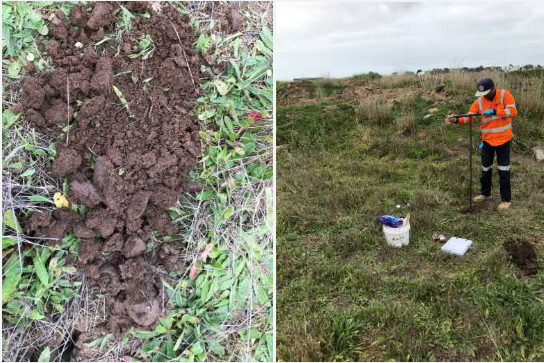
Plate 1: Hand augering within natural soils at HA01.
