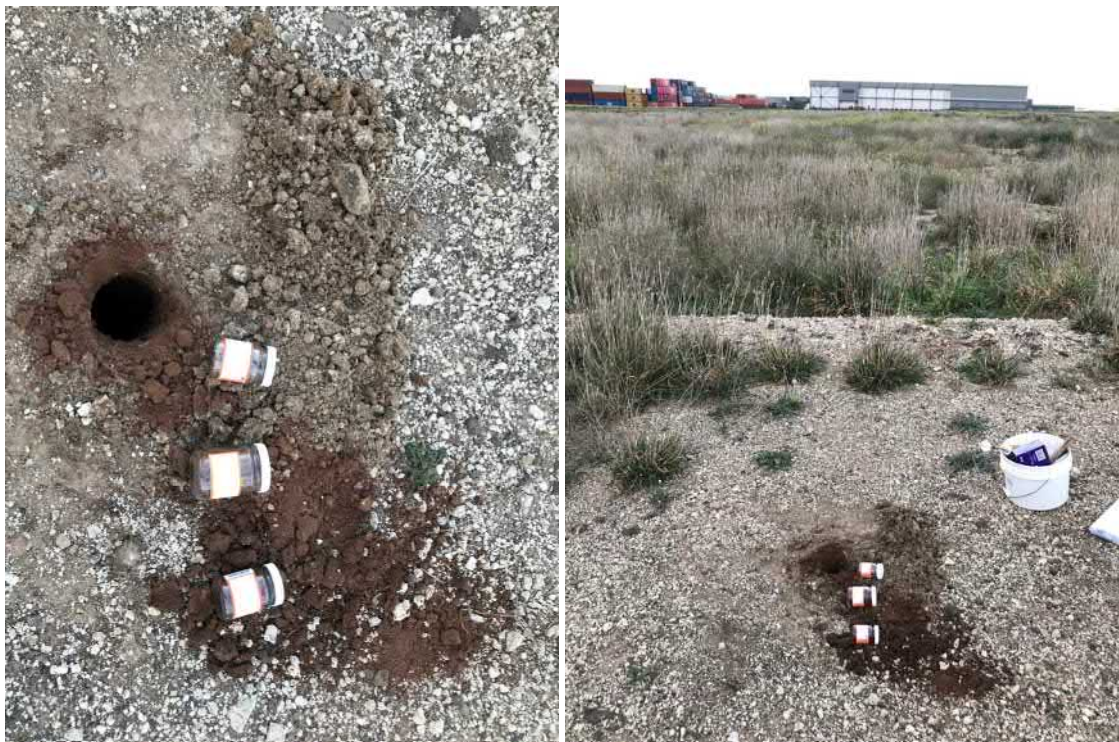
Plate 2: Hand augering through fill material to natural soil at HA03.
