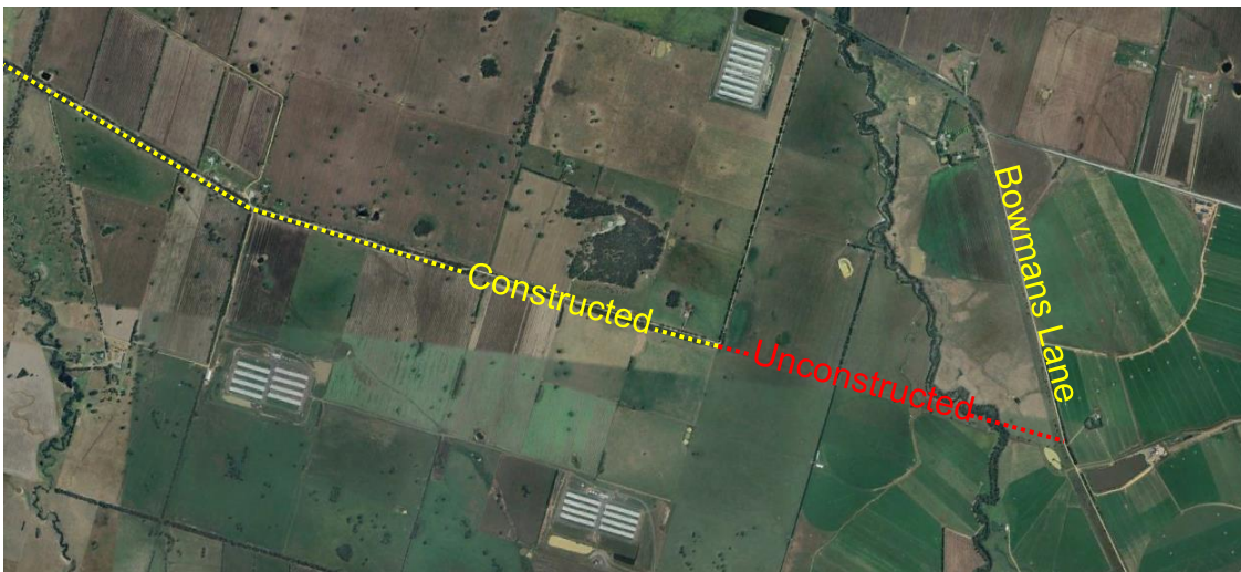
Diagram demonstrating the varying constructed elements of Graham Road (Source: Google Earth)
